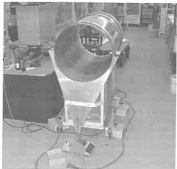
Fig. 7 The relative rollability apparatus, held at the Geography Department, University of Canterbury.
