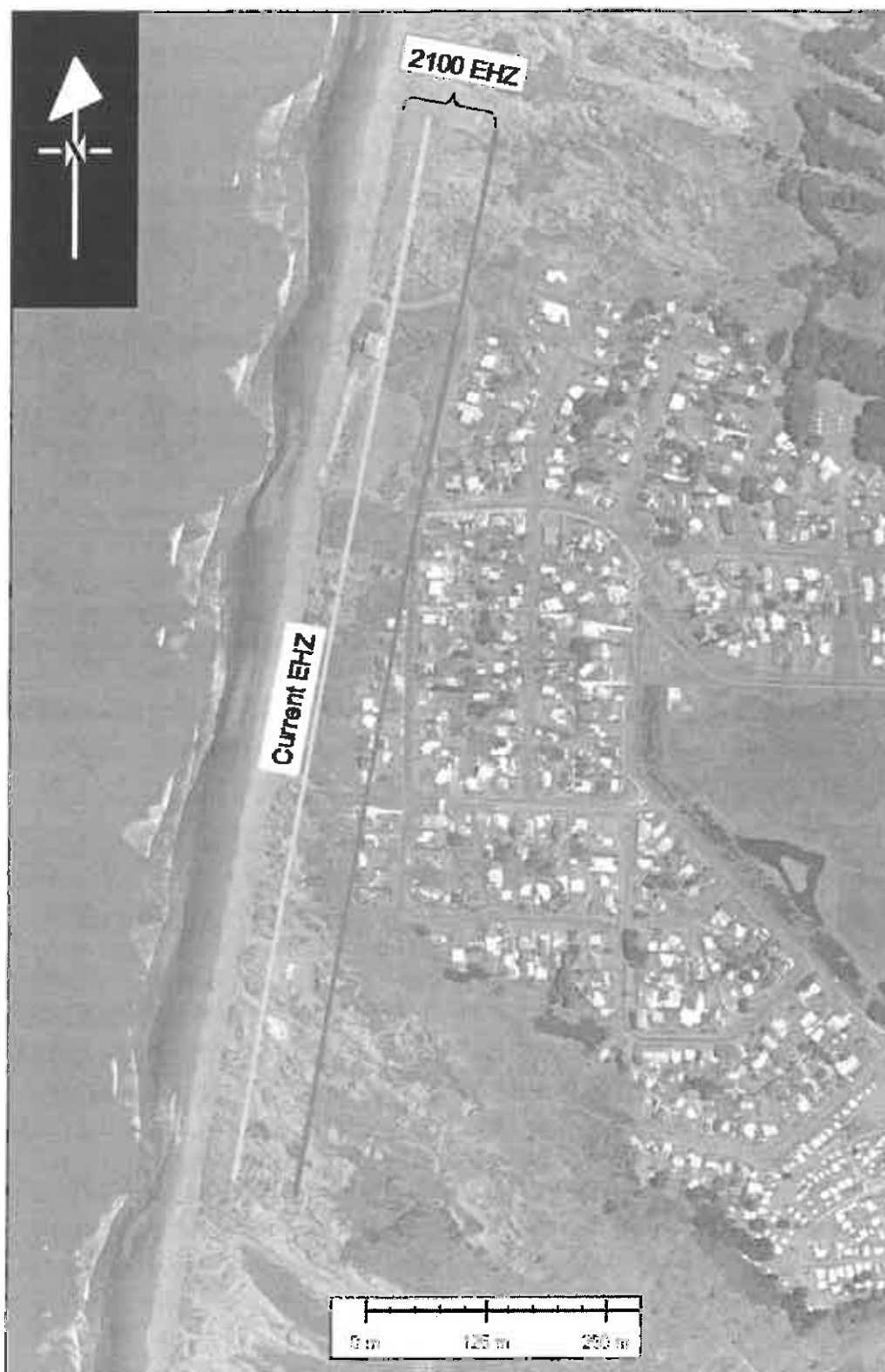
Figure 7 Erosion hazard zones for the current risk scenario and for the 2100 risk scenario.
