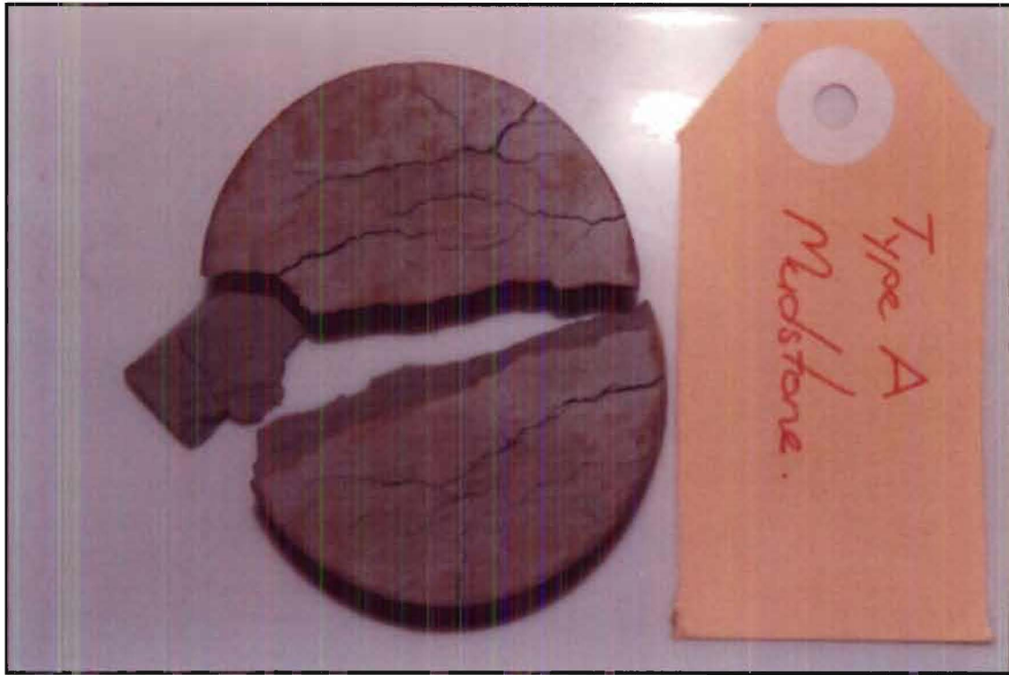
Figure 6.46 Type A sample after 20 wetting and drying cycles.
