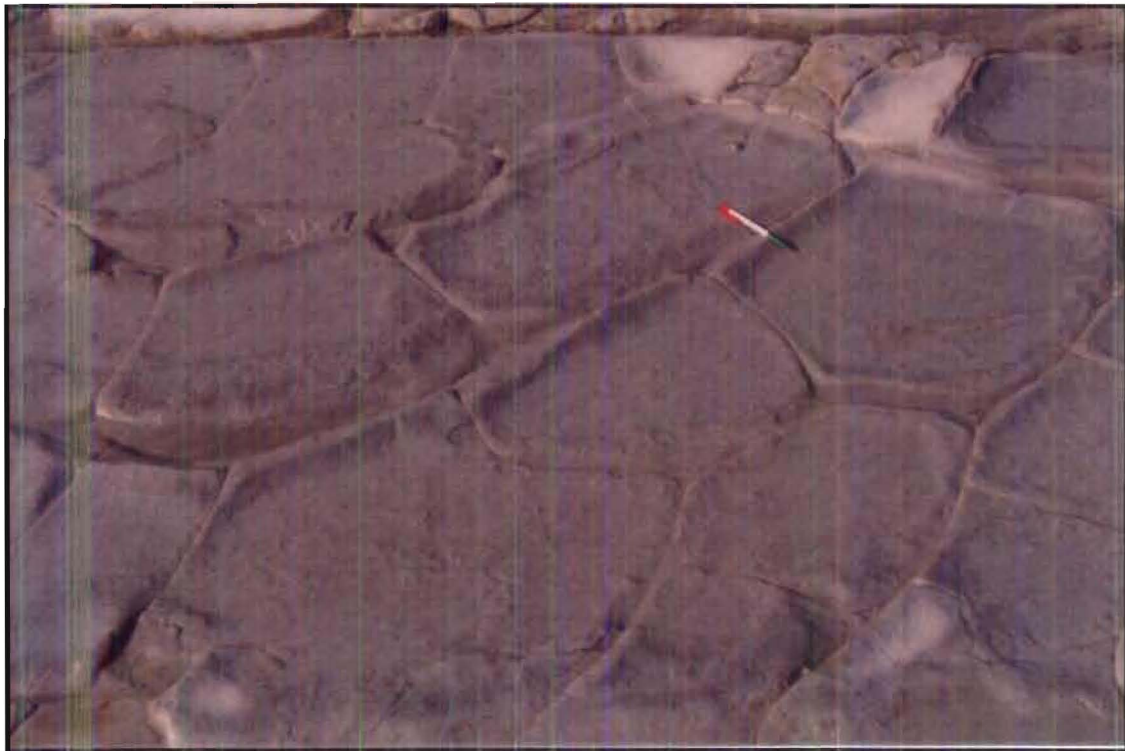
Figure 6.30 Water layering morphology with raised rims surrounding shallow pools of water at KM6 profile. Pen is 150mm long.
