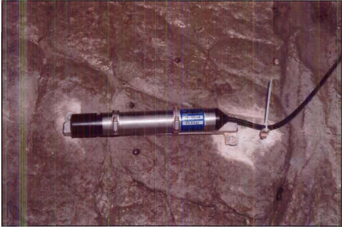
Figure 6.11 The Greenspan pressure transducer and cradle bolted to the platform at KM3. The transducer is 300mm long and 43mm in diameter.
