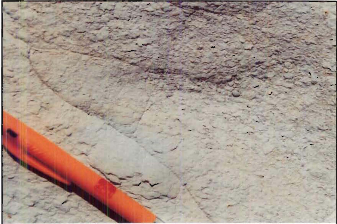
Figure 6.29 Pitted surface resulting from salt weathering. Viewable part of pen is 85mm long.
