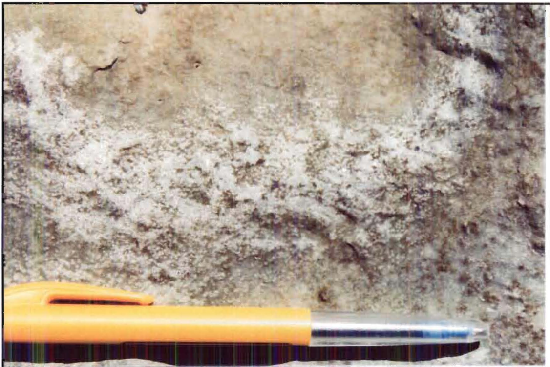
Figure 6.27 Salt crystal growth left after the pool of water has dried. Viewable part of pen is 120mm long.
