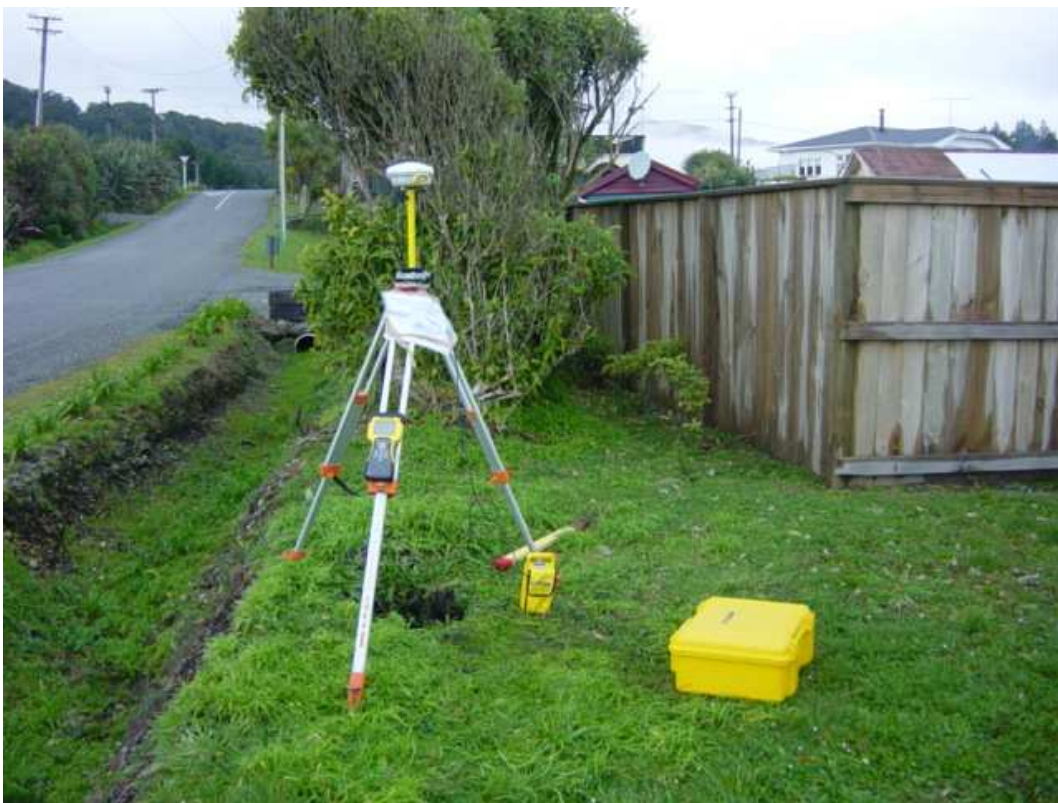
Figure 4.3 Trimble R8 and hand unit located on site above the benchmark
