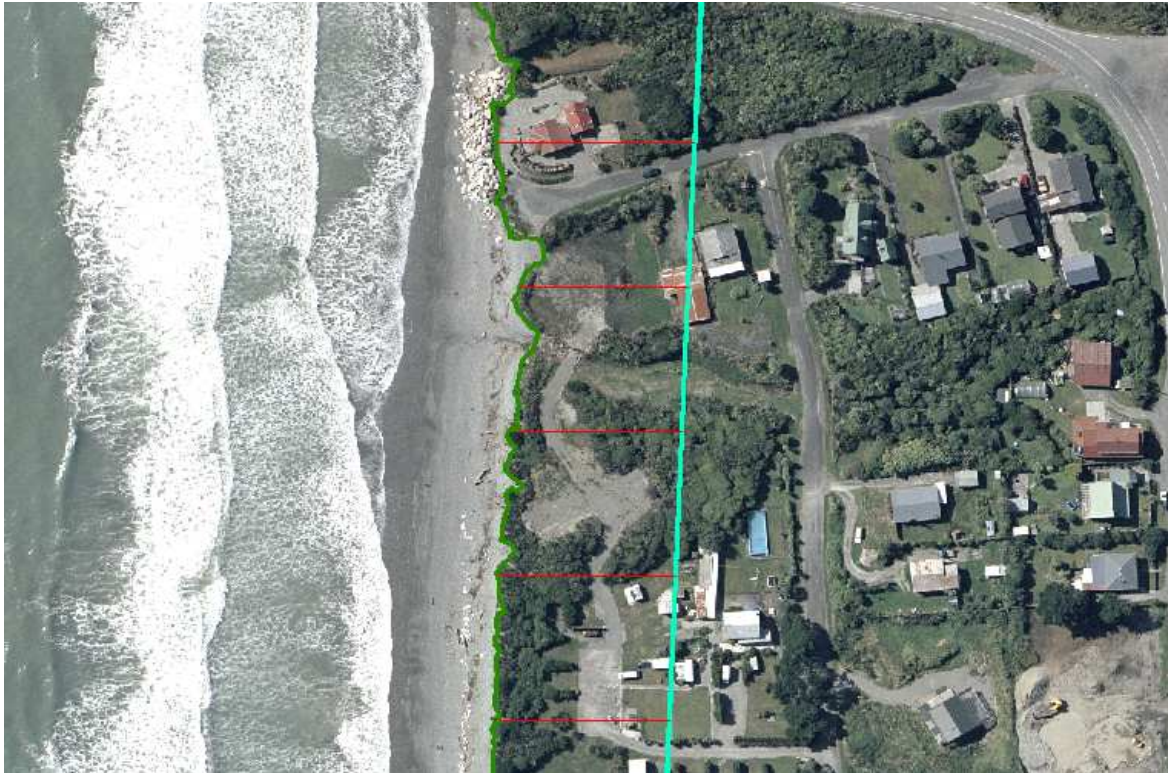
Appendix 3.3 Snapshot of ArcGIS displaying the process of measuring the perpendicular transects line for the vegetation line (2005).
