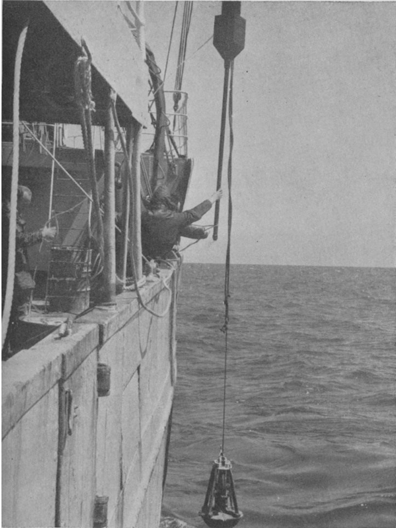
FIG. 3—Recovery of gravity corer with orange-peel grab acting as trip-weight.
