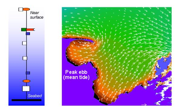
Data from instrument moorings provide calibration for computer circulation simulations – a cornerstone for understanding and predicting the physical and biological properties of these Bays. Instruments on the moorings measure temperature, salinity, tide height and currents. The computer simulation shows the interaction between Golden Bay, Tasman Bay and Cook Strait waters during the change between high and low tide.
