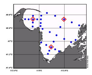
Fixed sites (blue) were sampled during ship surveys on four seasonal visits. Instrument moorings (red) sampled continuously. Additionally, when possible, a towed instrument (Biofish)<sup>5</sup> was used to sample while underway between sites, to provide a detailed picture of spatial variability.
