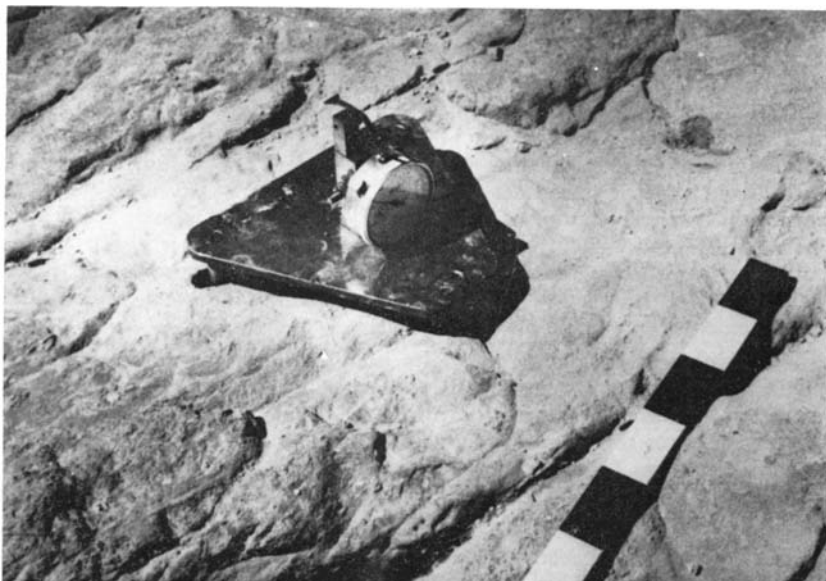
FIG. 6—Micro-erosion meter in place on a mudstone site. The dial-test-micrometer is mounted off-centre in the frame to provide three observations per site by rotation of the instrument. The gauge is provided with a lifter to avoid damage to the probe and the rock surface during placement. Scale interval: 5 cm.
