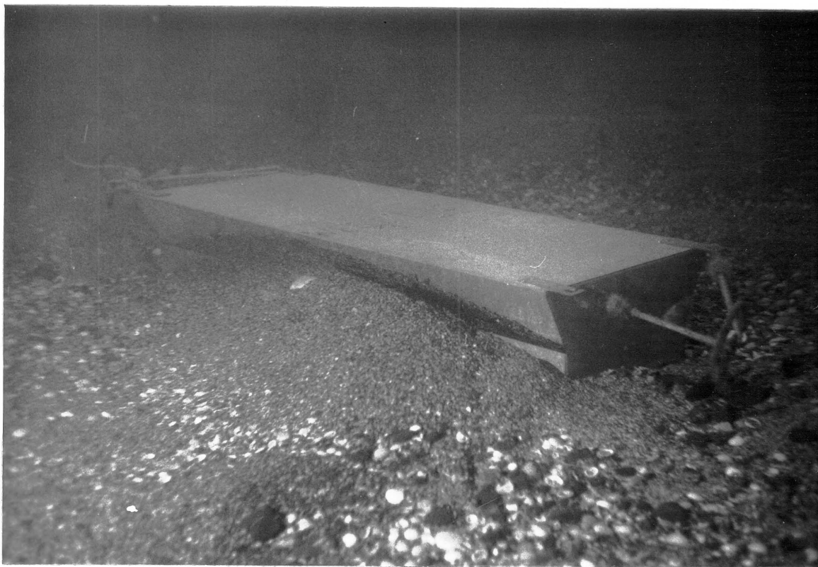
Plate 8.3 - One of the box sediment traps, viewed from the southwest. Note disturbance of natural dune morphology and the selective trapping of the finer (coarse sand) fraction of sediment.
