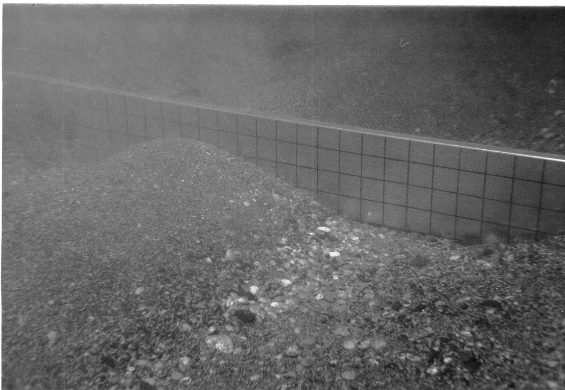
Plate 8.1 - Symmetrical dune bedform at 18 m depth in shelly, gravelly sand at Pataua. Dune height = 14 cm, wavelength = 100 cm. Each square division is 5 cm.
