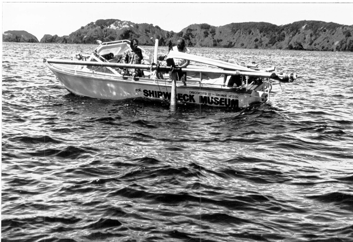
Plate 7.5 - Water hammer corer with 3 m long coring pipe extending toward the bow. The water hammer device is centrally located and is driven by water pressure through a 15 cm diameter hose from the boat's jet unit.
