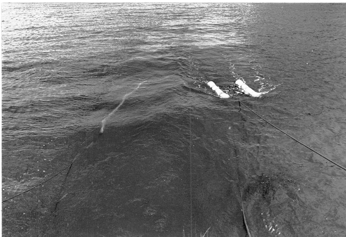
Plate 6.2 - Sub-bottom profiler equipment in tow. Boomer source on right with hydrophone eel on left.
