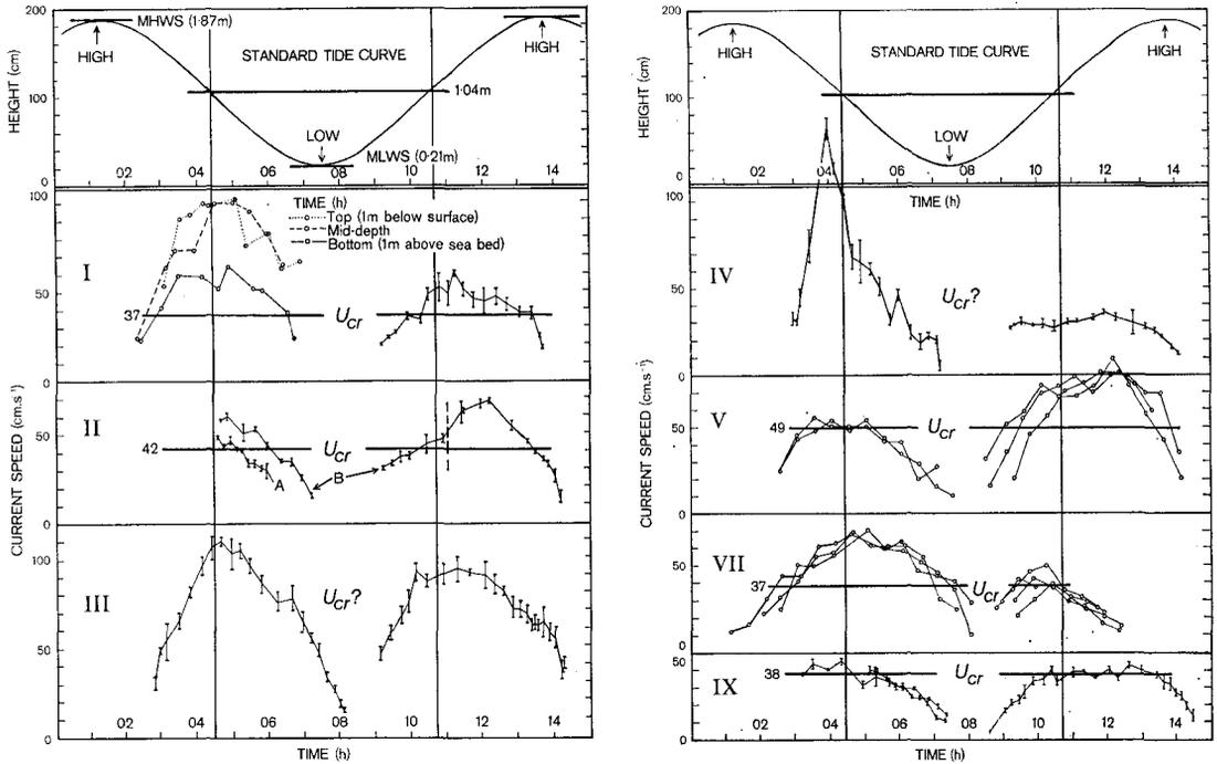
Fig. 3—Mean spring tidal currents (1 m above the harbour bed) as a function of time at seven oceanographic stations in Tauranga Harbour, 1974–75. Estimated critical erosion speeds ( $U_{cr}$ ) are superimposed on the plots.
