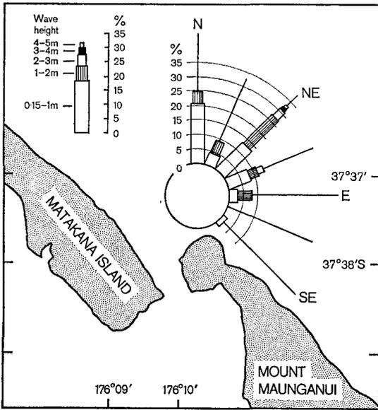
FIG. 4—Wave rose for the Tauranga Entrance showing the frequency of occurrence of various height classes and directions based on observations by Bay of Plenty Harbour Board pilots, 1974–75.
