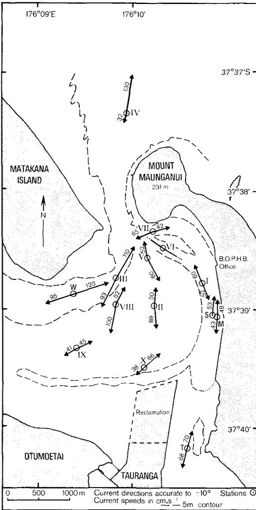
FIG. 2—Tidal current vectors at oceanographic stations for peak ebb and flood currents at mean spring tide, 1974-75.
