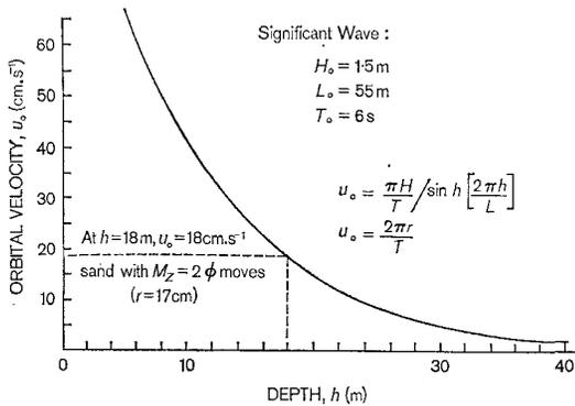
FIG. 6—Wave orbital velocity as a function of depth of water for the significant wave at the Tauranga Entrance.
