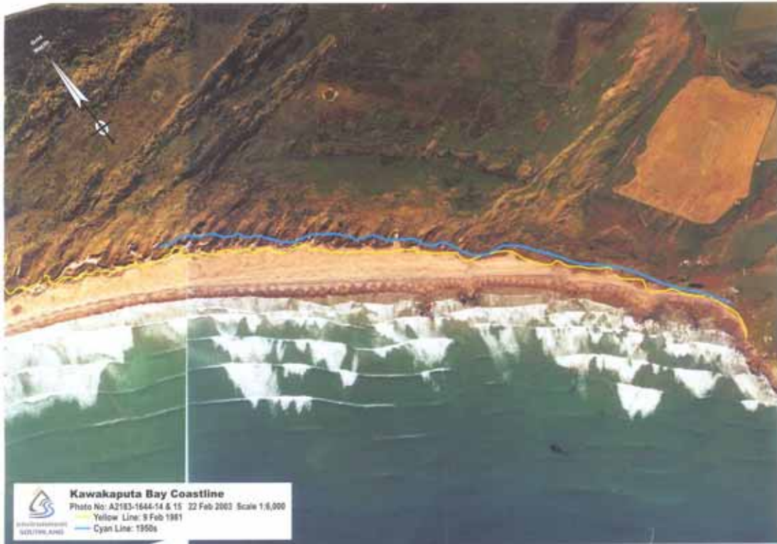
Figure 11 Coastline positions as of 1950 & 9 February 1981 overlaid on a 22 February 2003 photograph of the south east end of Kawakaputa Bay.
