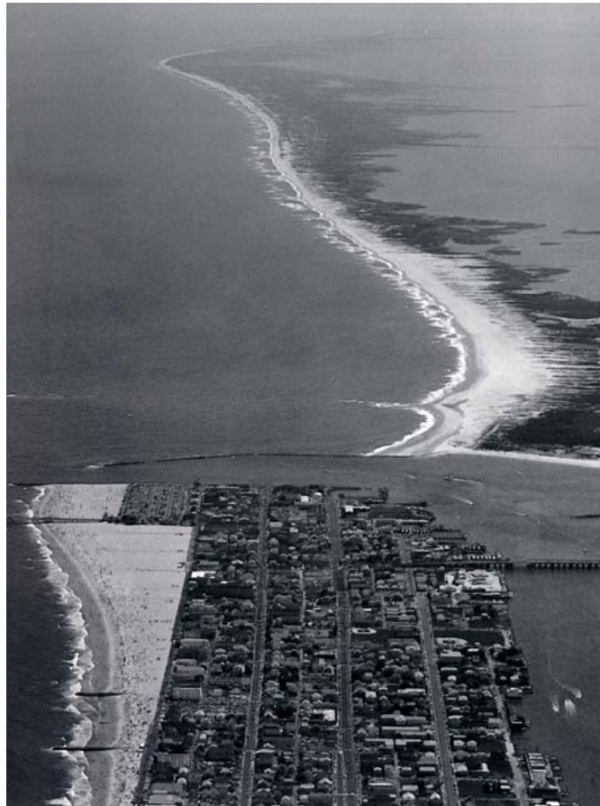
Figure 6-2 Shoreline changes resulting from the construction of jetties at Ocean City, Maryland. [from Komar (1998)]
