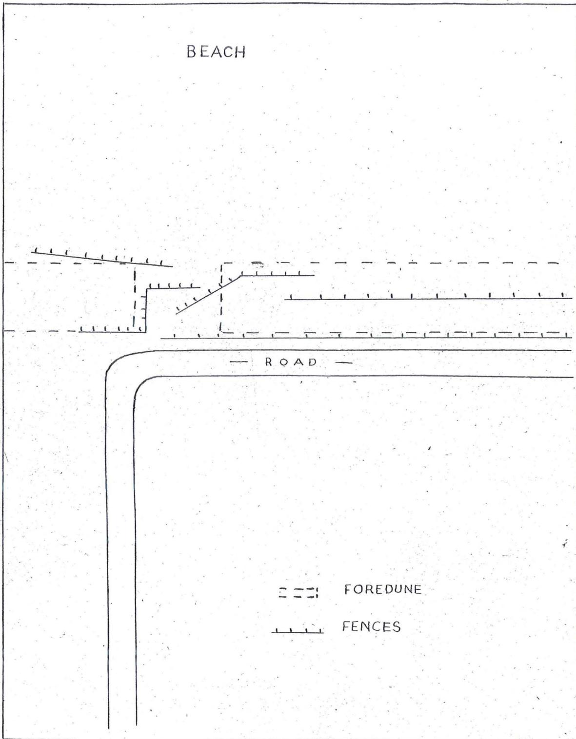
Fig. 32. FENCES COVERING A GAP IN THE FOREDUNE,
