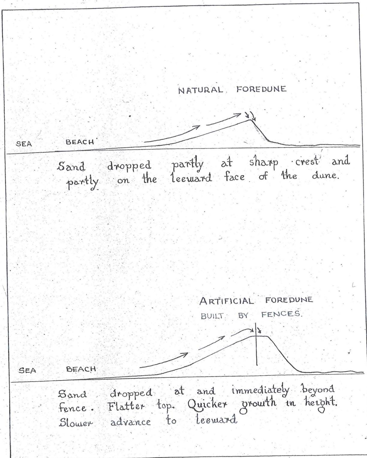
Fig. 19. THE SHAPE OF A NATURAL FOREDUNE COMPARED WITH THAT OF AN ARTIFICIAL FOREDUNE.
