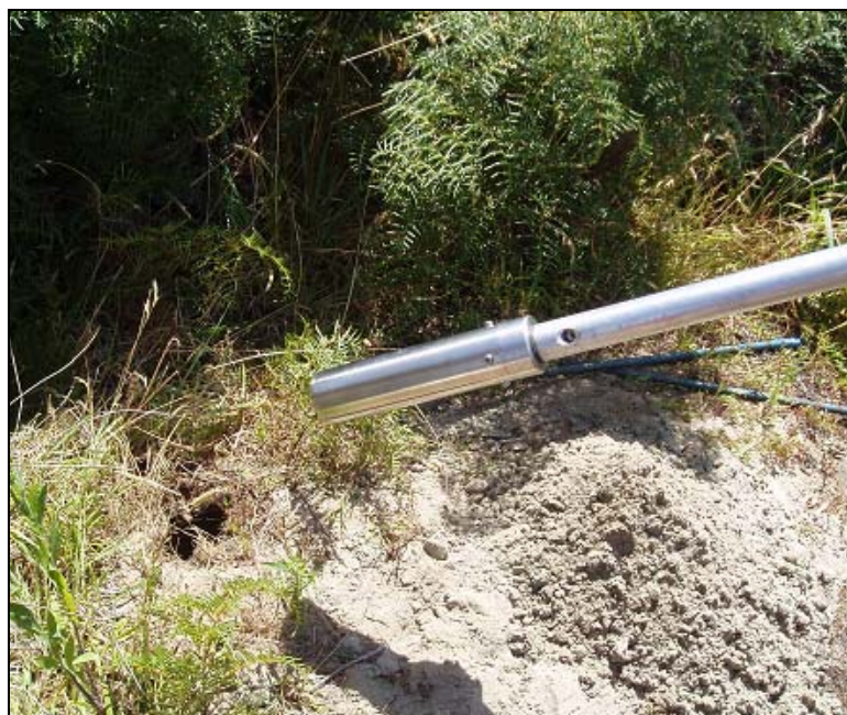
Figure 4.7: Stainless steel OSL tube attached to the auger shaft (Photograph: Helen Tribe, 2007).
