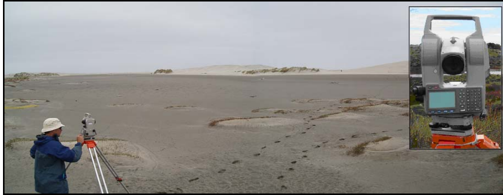
Figure 4.1: Surveying across Mullet Creek using a Sokkia SET 4010 EDM (detailed in inset) (Photographs: Helen Tribe, 2007).
