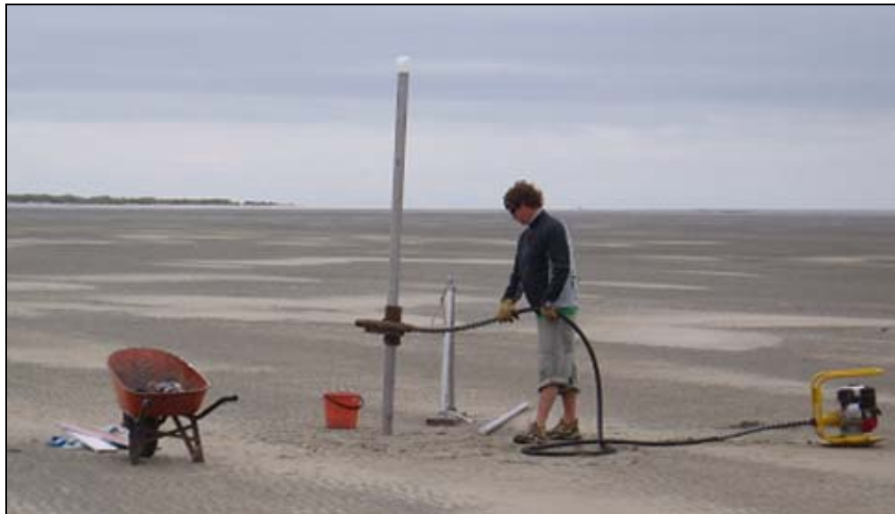
Figure 4.8: The vibracorer in use on the tidal flats of Farewell Spit. (Photograph: Helen Tribe, 2007).
