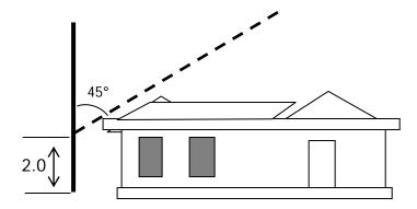
Figure 1: Daylighting Calculation
