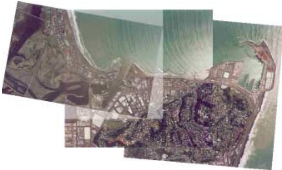
Figure 5.6. Aerial photo mosaic of the Port and Ahuriri Entrance showing wave refraction.
