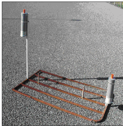
Figure 4.6. Example of a sediment traps mounted on a typical seabed frame
