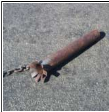
Figure 4.3. Flared pipe used for collecting surficial sediments.
