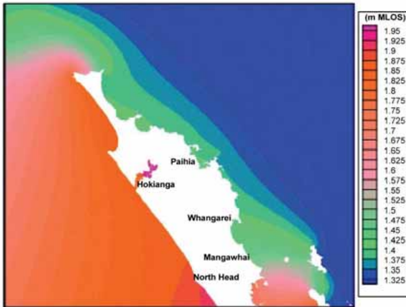
Figure 9: MHWS and Highest Astronomical Tide Above Mean Sea Level. Sourced from Bell & Gorman 2003 15
