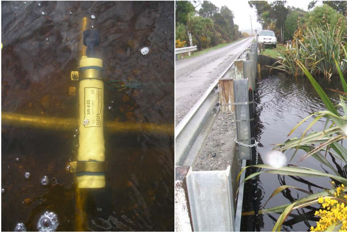
Figure 3.3. Water level recorders set up at the field sites. Left : short term XR-620-CTDm water level recorder in Totara Lagoon. Right : Long term CT2X water level recorder affixed to Waikoriri Bridge via a warratah.
