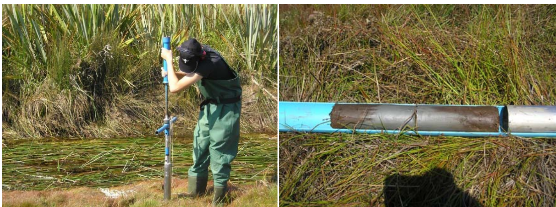
Figure 3.6. Left : Photograph showing the process of taking a sediment core from Shearer Swamp with a hammer corer. Right : Ejecting the core into a plastic tube following collection.
