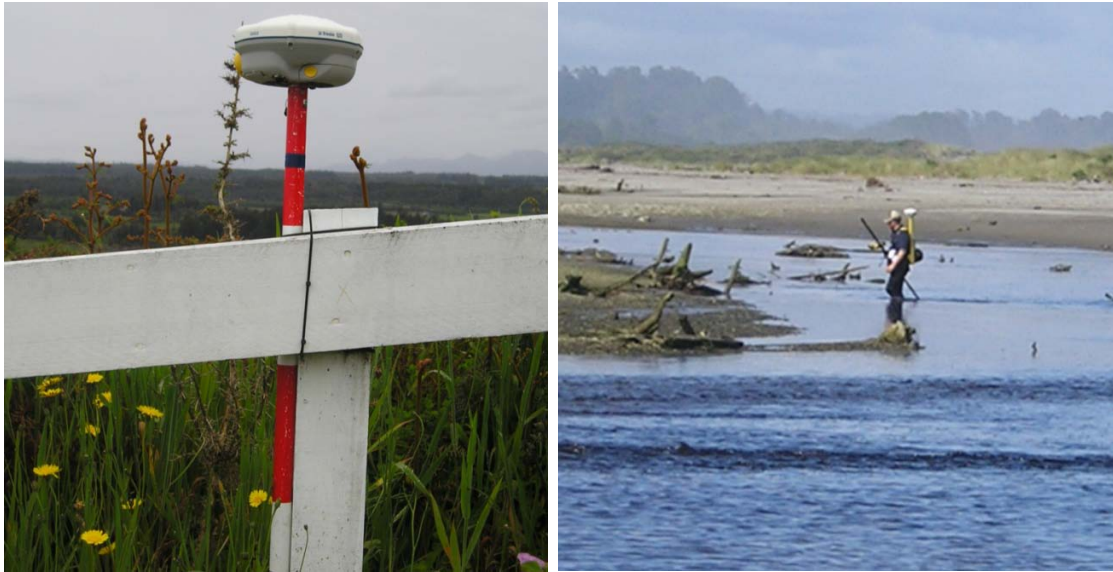
Figure 3.2. Left : Base station receiver set up at Ross Cemetery. Right : Surveying the river mouth end of Totara Lagoon.
