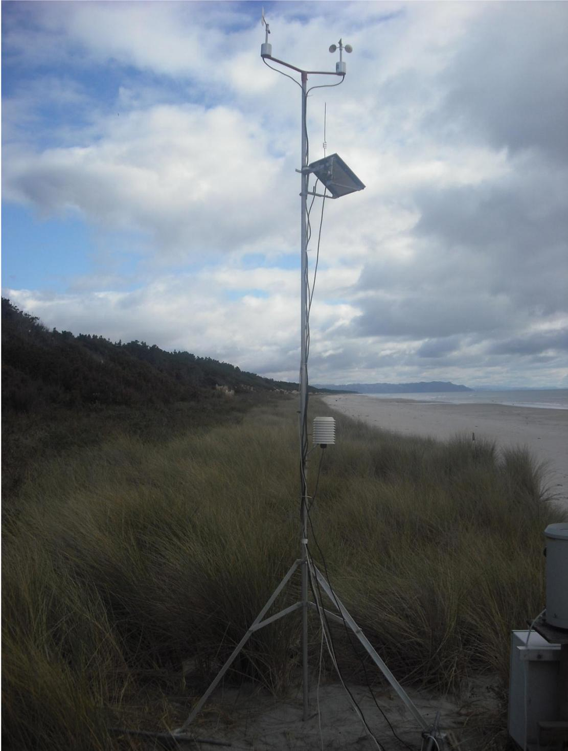
**Figure 4.1:** Station set-up at sample site A measuring wind speed, direction and rainfall. Wind speed and rainfall are collected from the top of a 4m tower.
