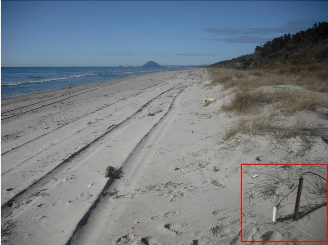
**Figure 4.3:** Piezometer placement in the fore dune of Station B. Red box indicating position of PVC tubing, pressure sensor and waratah.
