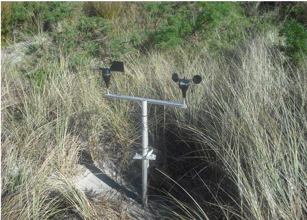
**Figure 5.3:** Wind instruments at sample site B sampling wind speed and direction at average plant height (0.8 m).
