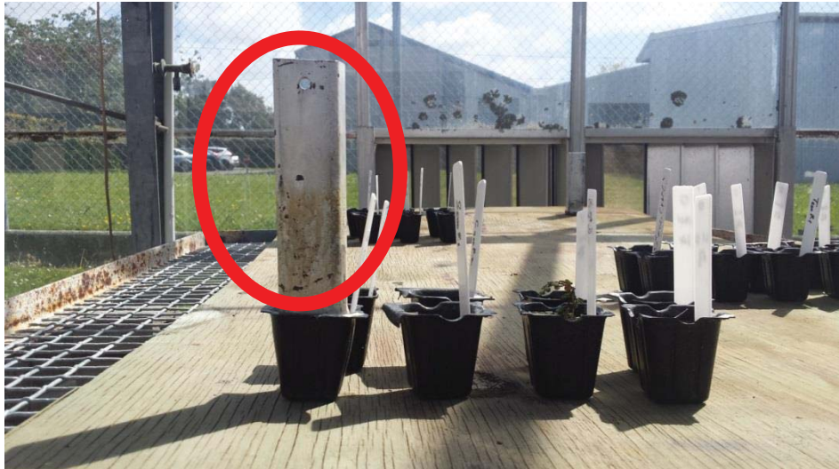
Figure 3: The tamping experimental setup and the tamping "foot" (circled in red) that was used. The weight is placed on one of the plants and the other replicates can be seen.
