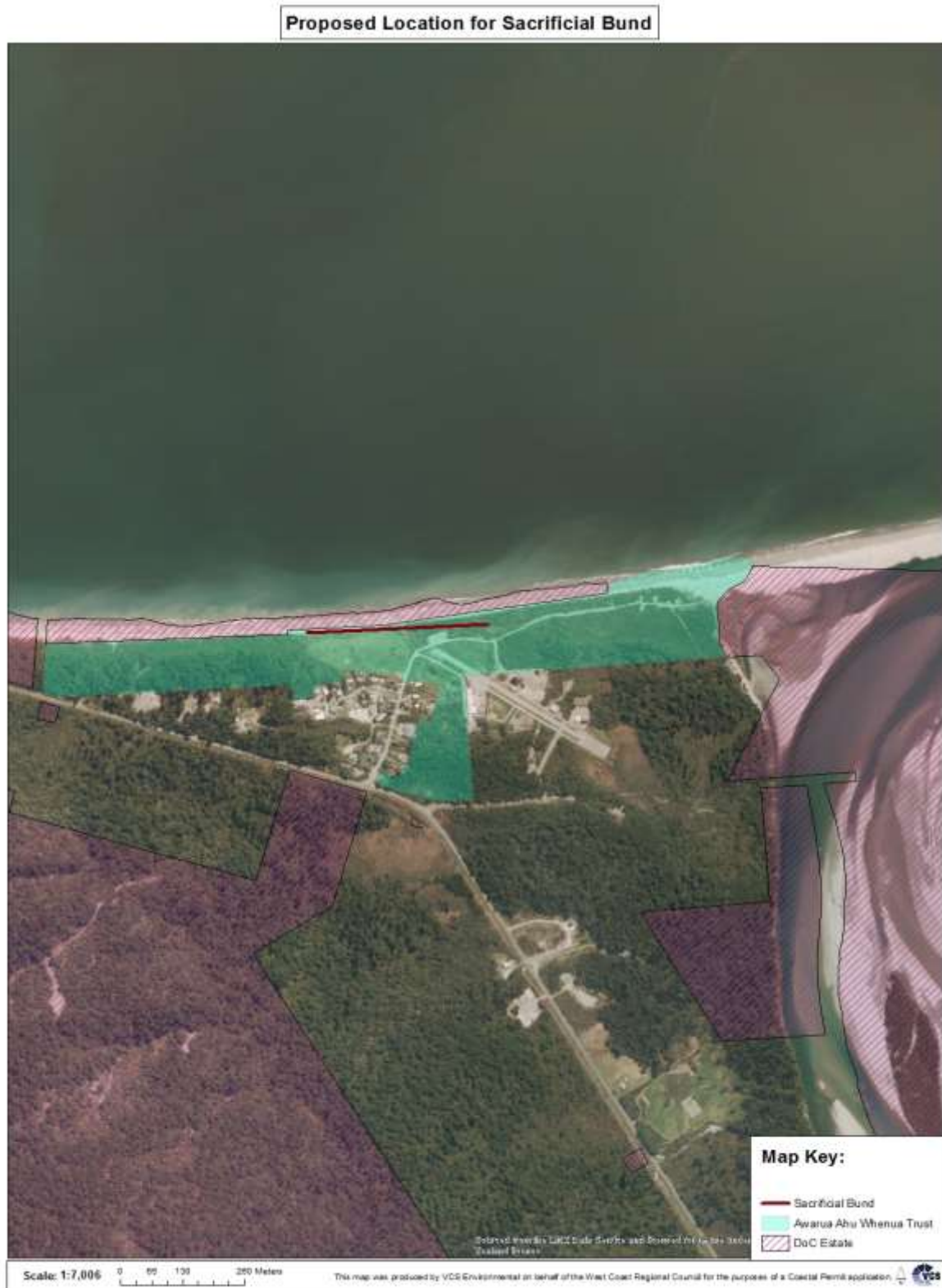
APPENDIX A. AERIAL PHOTOGRAPH SHOWING THE PROPOSED LOCATION OF THE SACRIFICIAL BUND
