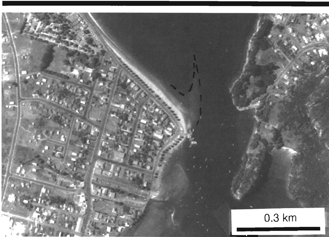
Figure 7. 'Low-angle half-delta' at Whitianga Inlet. Note the low angle of the inlet channel with respect to the barrier shore, and the ebb delta restricted to a small sand bar on the inner bank of the channel.
