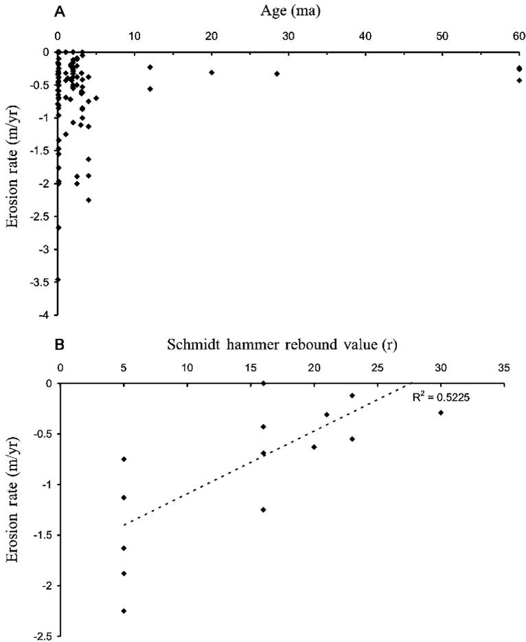
**Fig. 5** The relationship between erosion rates derived by Gibb (1978) and **A**, lithological age and **B**, rock hardness. Lithological age is determined by the latest geological mapping and rock hardness from field strength testing as part of this investigation. See Table 1 for details.
