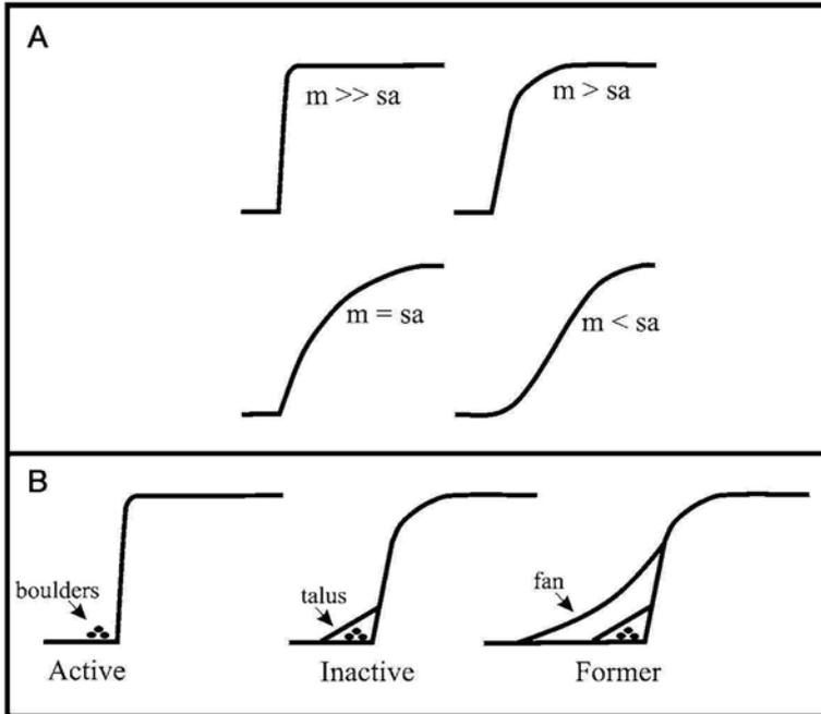
**Fig. 2** A, A classification of cliff profiles based on the relative efficiency of erosive processes ( $m$  = marine erosion,  $sa$  = subaerial erosion); B, cliff profile development through increasing abandonment by the sea. Modified from Emery & Kuhn (1982).
