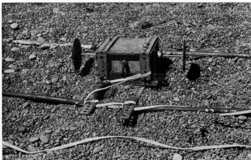
FIG. 4.—Dynamometer mounted on conduit frame for velocity measurements near the bed.
