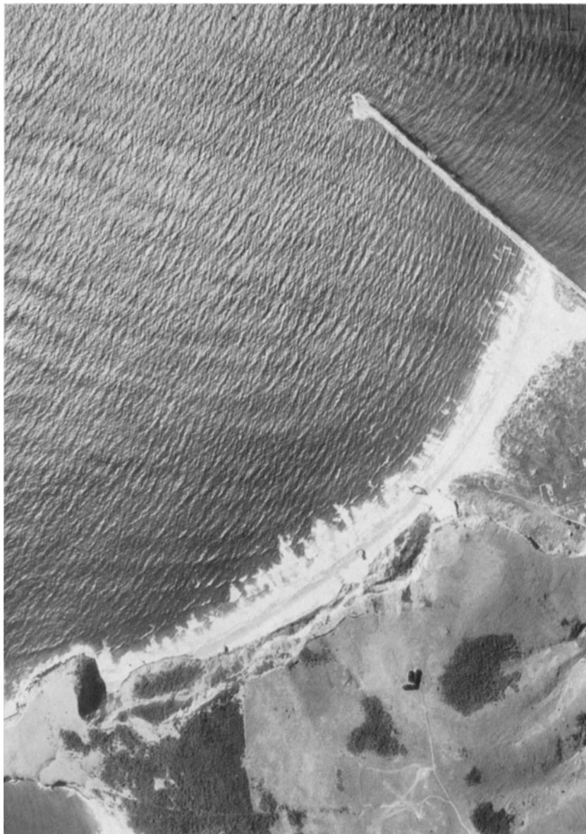
FIG. 6—Interplay of north-easterly sea and refracted southerly swell off the mouth of Otago Harbour. Scale approximately 25 chains to an inch. (North in the photo is to the left above, the mole extending north-east.)
