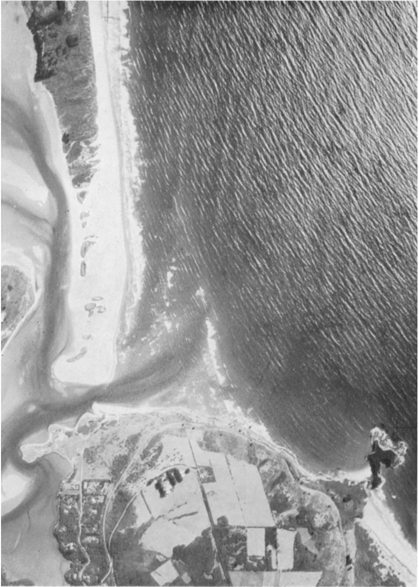
FIG. 7—The influence of sea and swell in forming breakers on Warrington Spit can be seen from the spacing between breakers in the surf zone. Scale approximately 25 chains to an inch.
