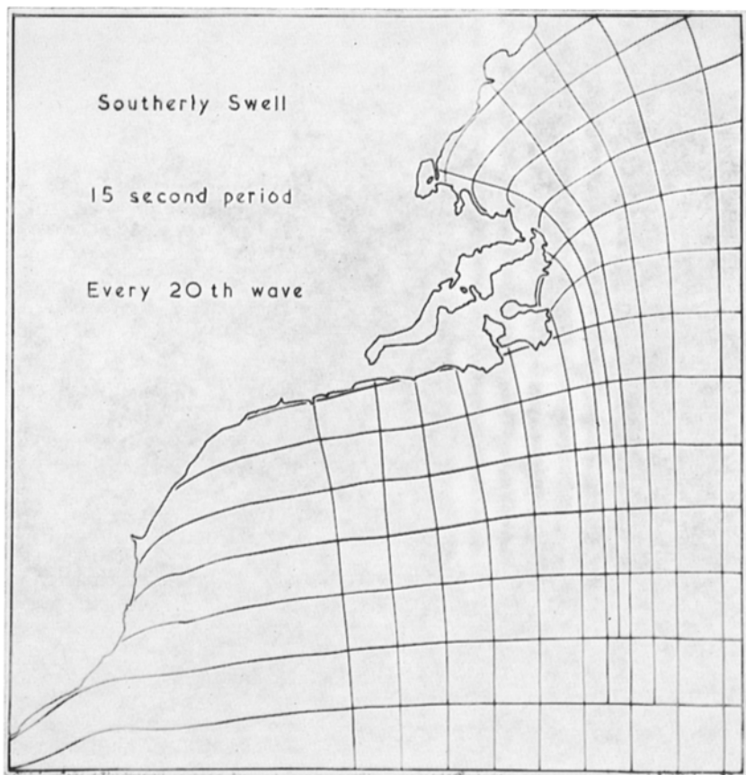
FIG. 4—Refraction diagram for a southerly swell of 15 sec period. Orthogonals, equally spaced in deep water, indicate the amount of attenuation undergone by the wave fronts during refraction. Such attenuation is accompanied by a decrease in wave height.
