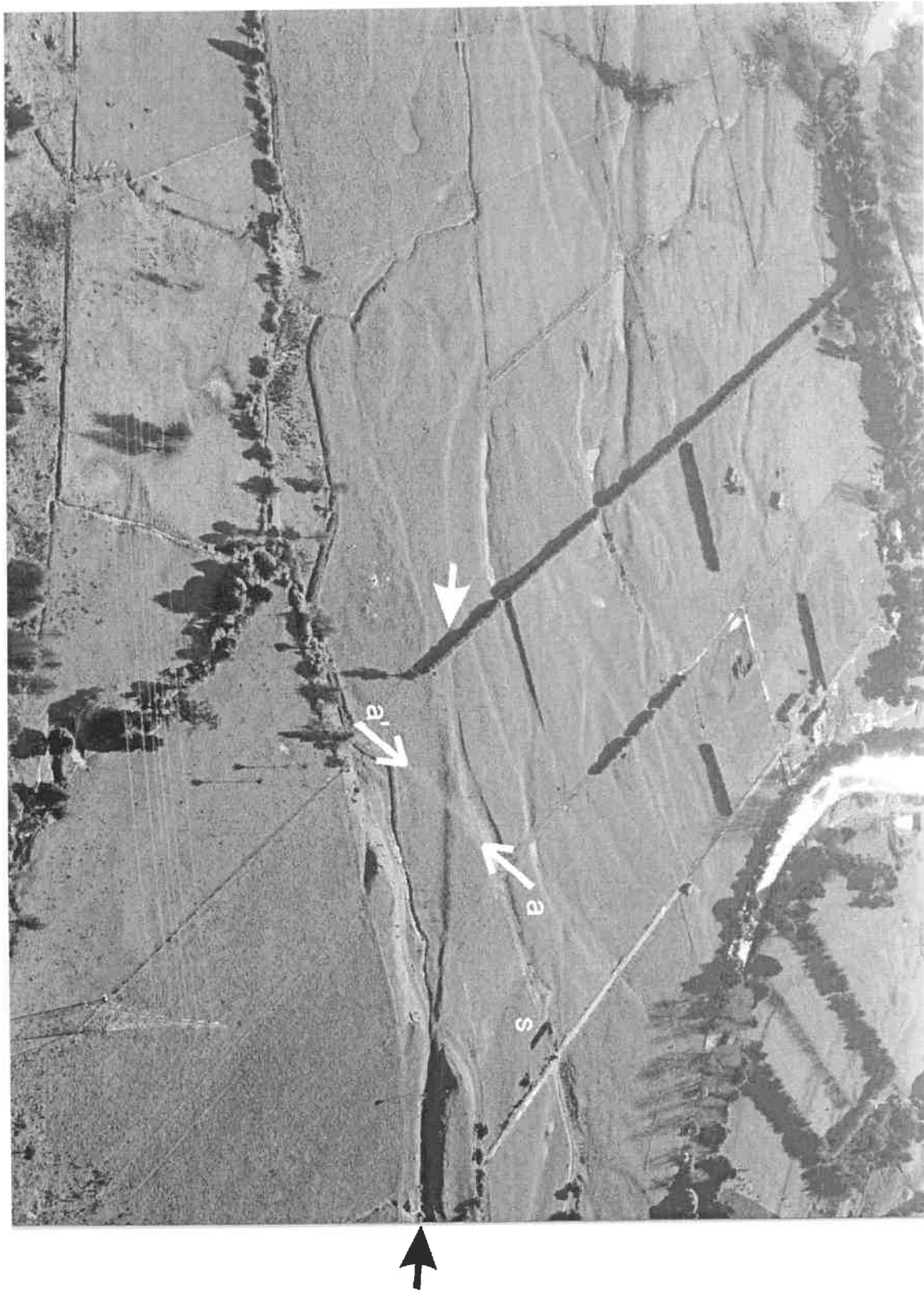
Fig. 10. Aerial photograph looking north-northwest across northeast-trending Northern Ohariu fault, Florida Road/Ohau River area. Bold arrows show fault's location. The 3.0-3.5 m net displacement of the young terrace riser is denoted by the arrows labelled a-a', and is interpreted to represent the amount of surface rupture displacement that occurred at this site during the most recent earthquake. "s" is location of silage pit discussed in text. Photo: D.L. Homer, Institute of Geological & Nuclear Sciences (photo ref. CN 39576 17).
