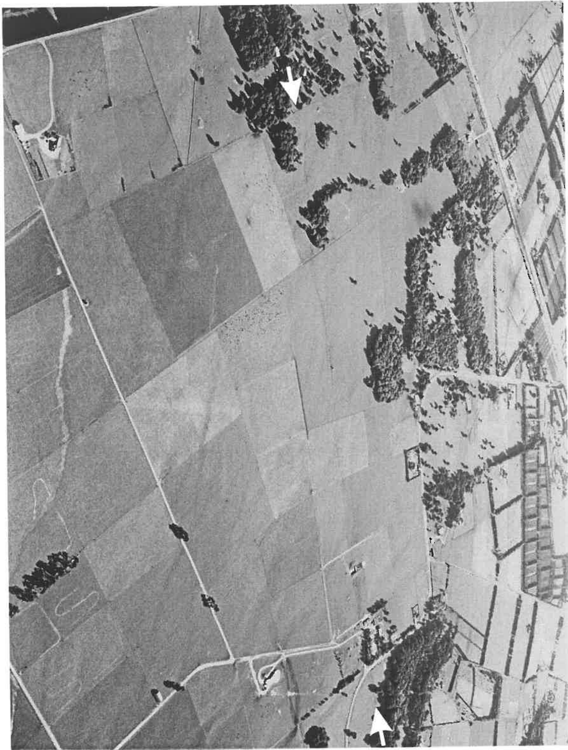
Fig. 4. Aerial photograph looking northwest across the northeast-trending scarp, 1-2 m high, of the Northern Ohariu fault, Te Horo/Old Hautere Road area. Bold arrows show the location of the fault which extends left to right across middle of photo. State Highway 1 runs diagonally across upper-left of photo, and Old Hautere Road is at upper-middle left. The extensive alluvial terrace in the photo that is displaced by the fault is predominantly Ohakean in age (about 10 000-15 000 years old).
