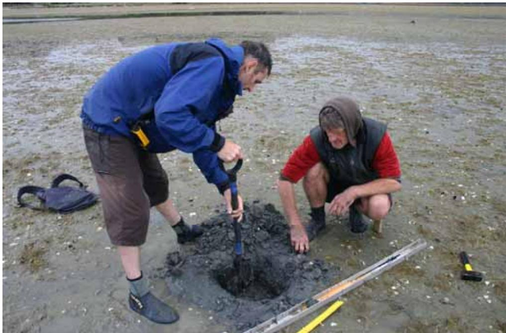
Figure 6.4: Installing a sedimentation plate in the Pauatahanui Arm of the Porirua Harbour. The depth to each sediment plate will be measured each year, allowing the sedimentation rate to be determined.
