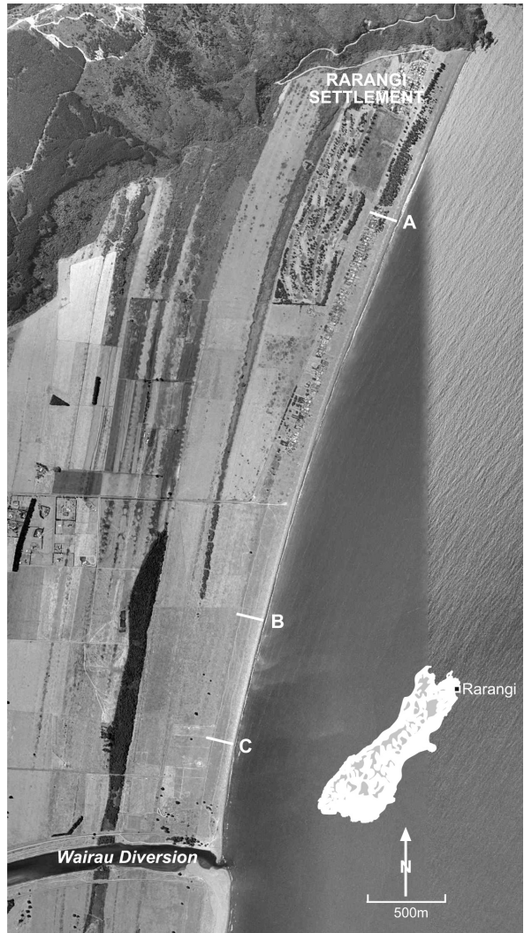
Figure 6 – Location of the three traverses from Rarangi. Traverse ‘A’ is located in an area of significant groundwater abstraction, while traverses ‘B’ and ‘C’ are across areas where the groundwater is ‘undisturbed’.
