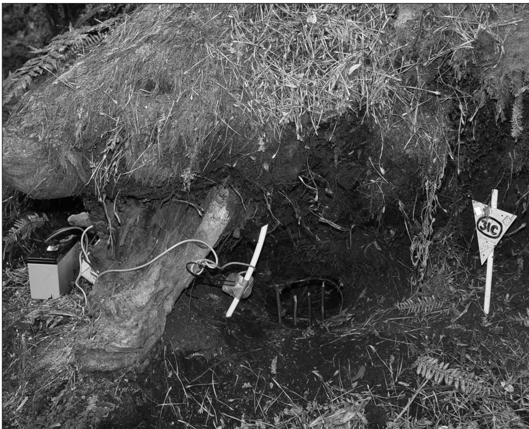
Figure 2. PIT tag recorder set up at a taiko burrow. Note the antenna layout around the burrow entrance and stick fence, motion sensor on stake, white PIT tag recorder box housing the RFID reader and datalogger (partly obscured), wire cables and 12-volt battery. The recorder unit and wires are normally covered with vegetation to stop taiko dragging cables into the burrow. Photo: GA Taylor
