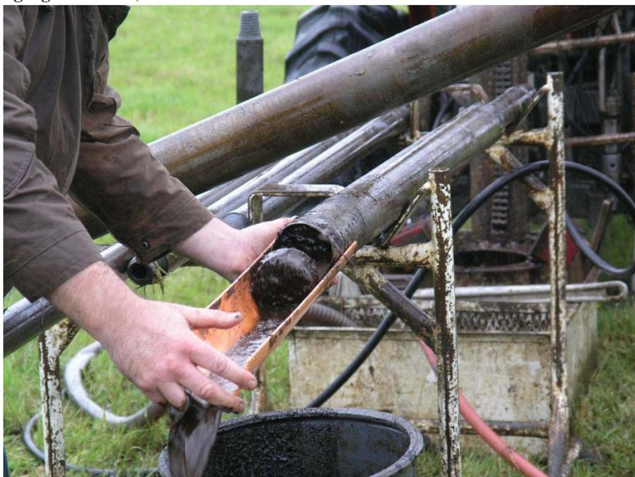
Figure 34(b). Water extrusion of core from bore casing, 2008.
