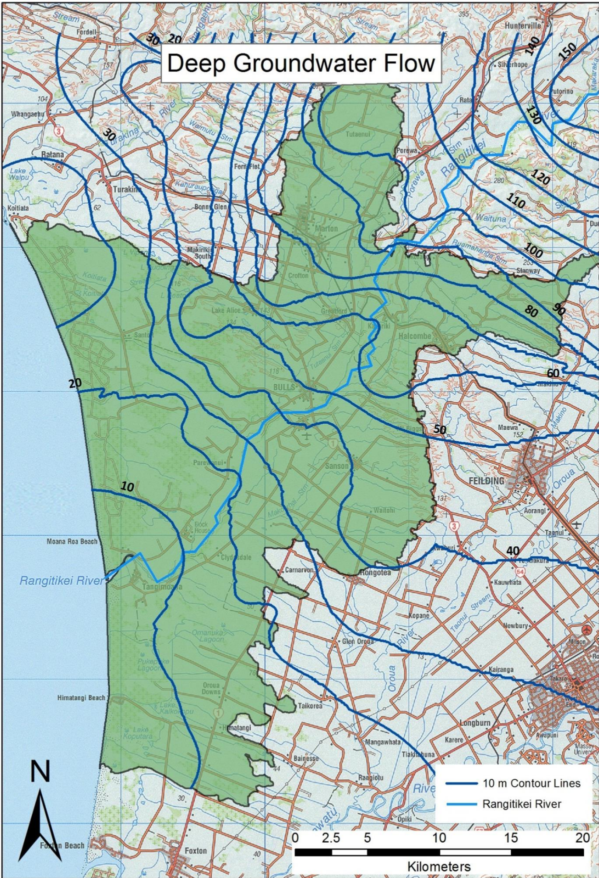
Figure 24: Deep groundwater flow from wells screened greater than 30 m deep. Contours are masl.
