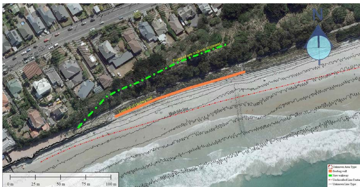
Figure 1 Showing the likely extent of the proposed geotube wall and the possible location of a relocated pathway
