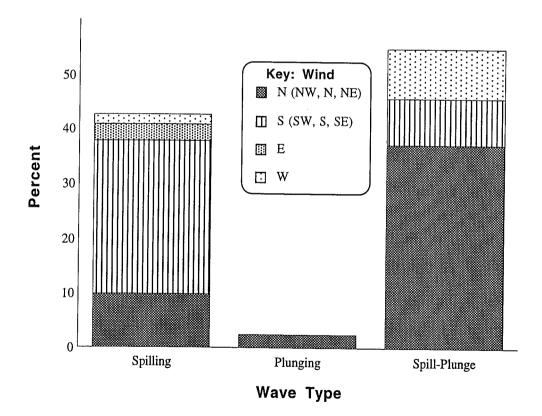
Fig. 4.20: Observation breaker type distribution with respect to wind direction at the time of observation.
