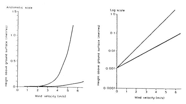
Fig. 3.3: Velocity profiles over a bare sand surface, (left), and the same profiles plotted on a logarithmic height scale, (right). (source; Pethick, 1984).
