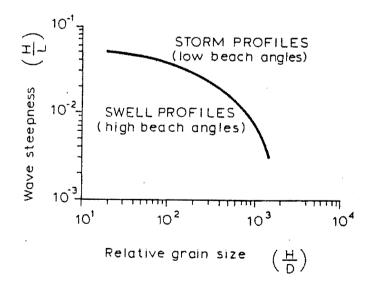
Fig. 5.50: The critical wave steepness required for the transition from swell to storm profiles is dependent on the relative grain size of the beach sediments in relation to the wave height. (after Iagaki & Noda, 1963; in Pethick, 1984)
