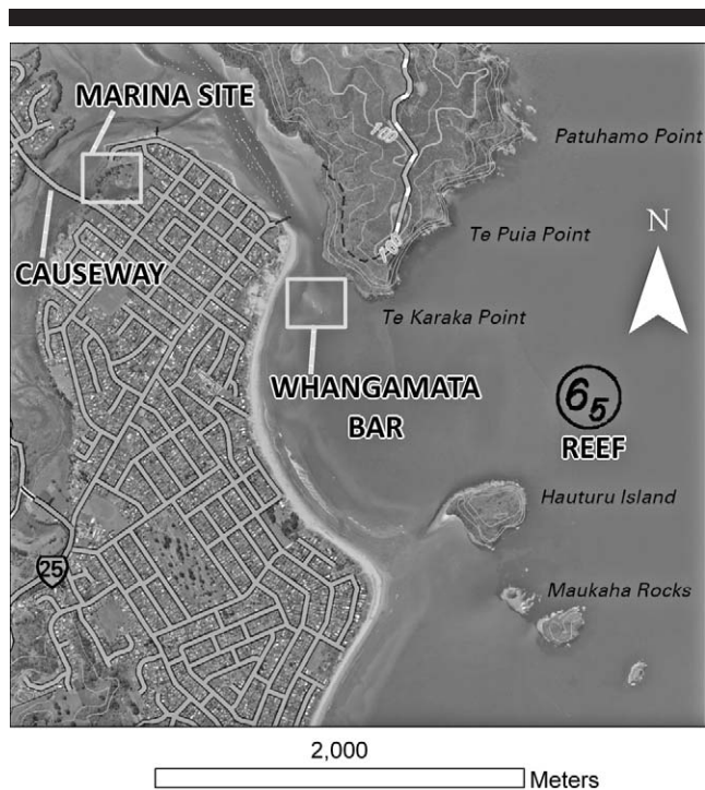
Figure 17. Location of the Whangamata Bar surfing break, proposed marina, offshore focusing reef (shoals at 6.5 m from 12 m deep), and harbor inlet. (Background map stream over the Internet from ArcIMS geographic data server of Land Information New Zealand.)
