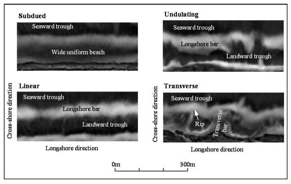
Figure 3 Examples of morphologies corresponding to the 4 configuration classes derived in the text.
