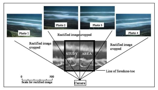
Figure 2. An example of a panorama of 4 time-exposure photographs (above), and the corresponding rectified and merged images (below). Areas of high intensity represent elevated features such as sand-bars, and the intermediate areas of low intensity represent rip channels and longshore troughs Two hundred metre wide segments of rectified image have been retained at the longshore margins of the 500 m long study site to assist in the interpretation of 3D structures.
