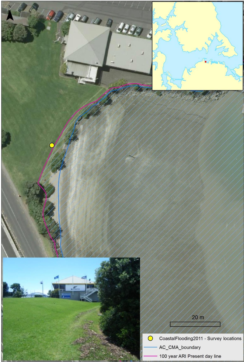
Figure 8-13: Verification of present-day 0.01 AEP (100-year ARI) storm-tide line against surveyed location of maximum flood incursion during 23 Jan 2011 storm-tide, at St Marys Bay.
