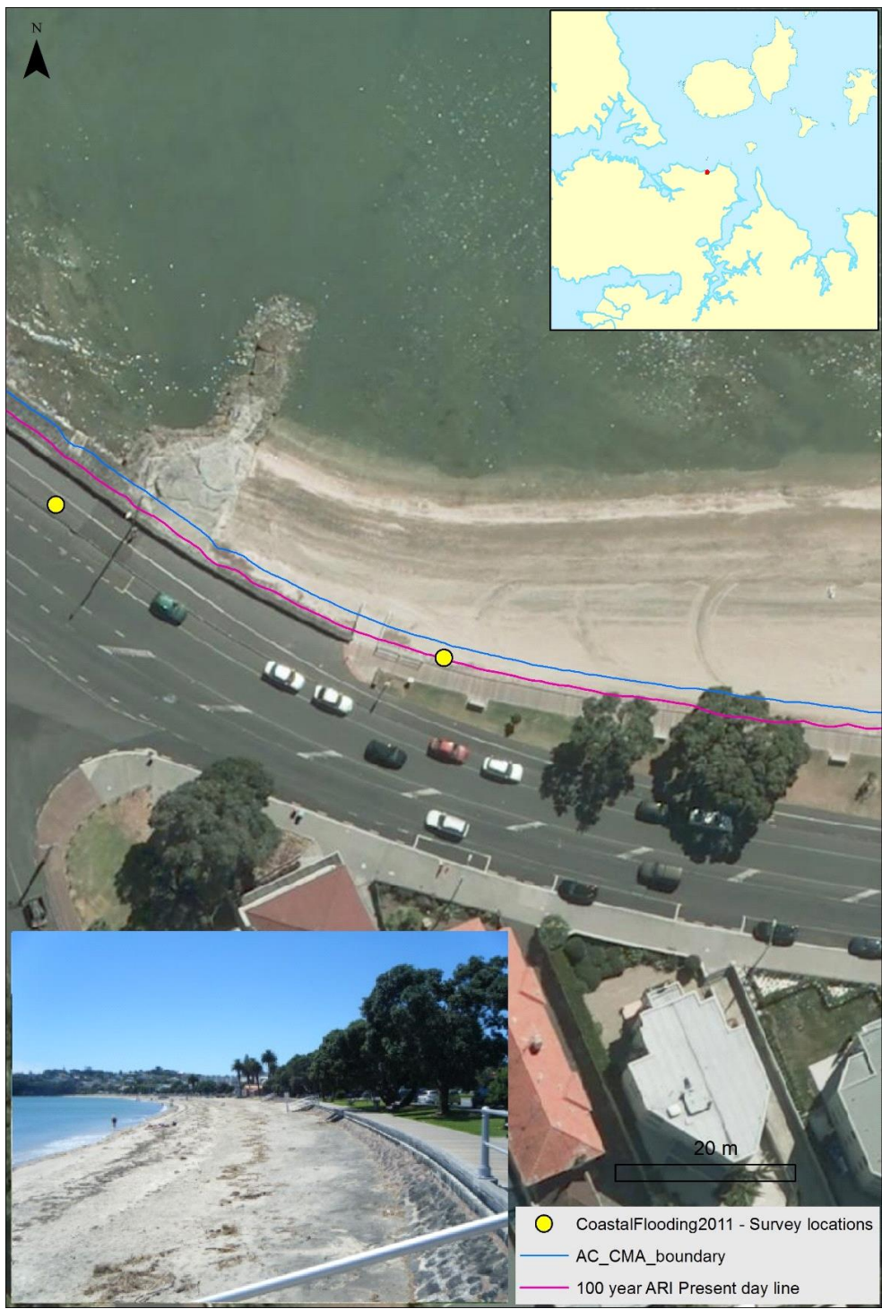
Figure 8-11: Verification of present-day 0.01 AEP (100-year ARI) storm-tide line against surveyed location of maximum flood incursion during 23 Jan 2011 storm-tide, at St Heliers Bay.
