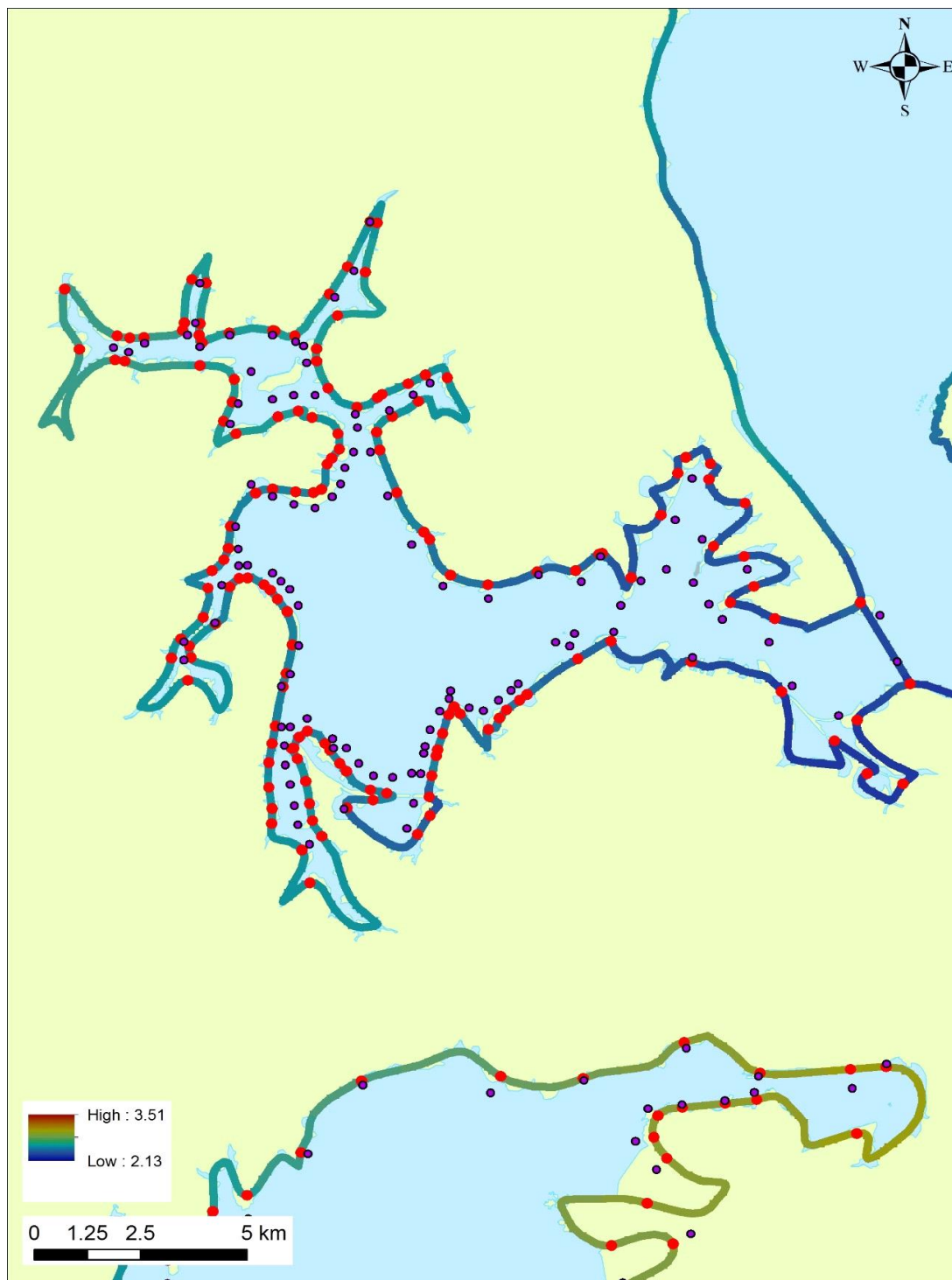
Figure 8-3: Map of Waitemata Harbour with interpolated elevation values on the simplified coastline.
