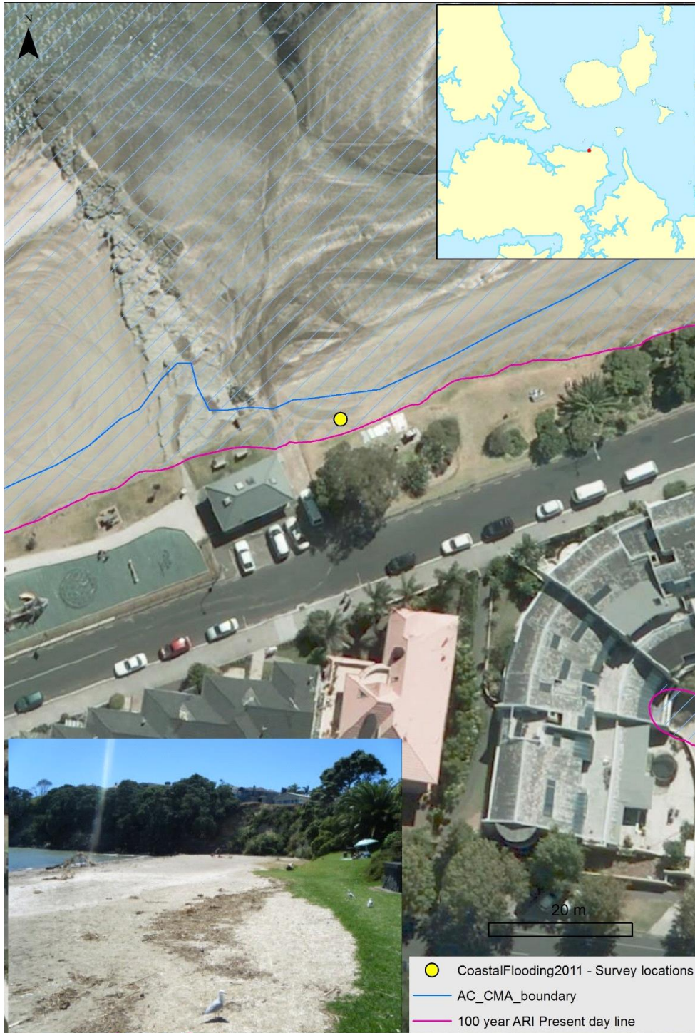
Figure 8-12: Verification of present-day 0.01 AEP (100-year ARI) storm-tide line against surveyed location of maximum flood incursion during 23 Jan 2011 storm-tide, at St Heliers Bay (east).
