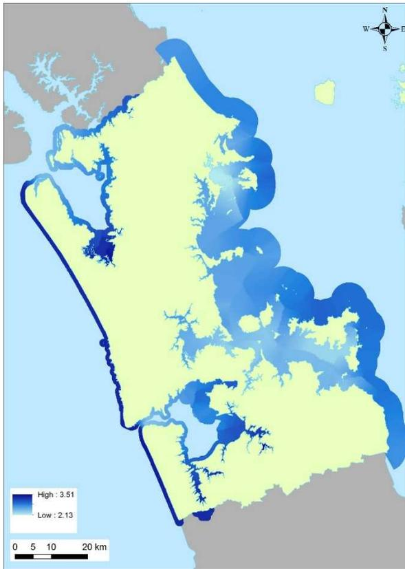
**Figure 3-4: Map of Auckland region with water surface for 0.01 AEP (100-year ARI) elevations.**
