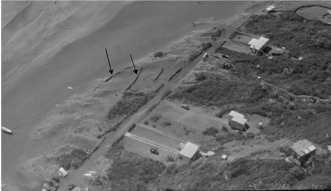
Figure 6: Photograph of Piha taken in January 1951 to the immediate north of the surf club showing brush fences (examples arrowed) erected to control wind erosion. (Whites Aviation photo – from Alexander Turnbull Library).
