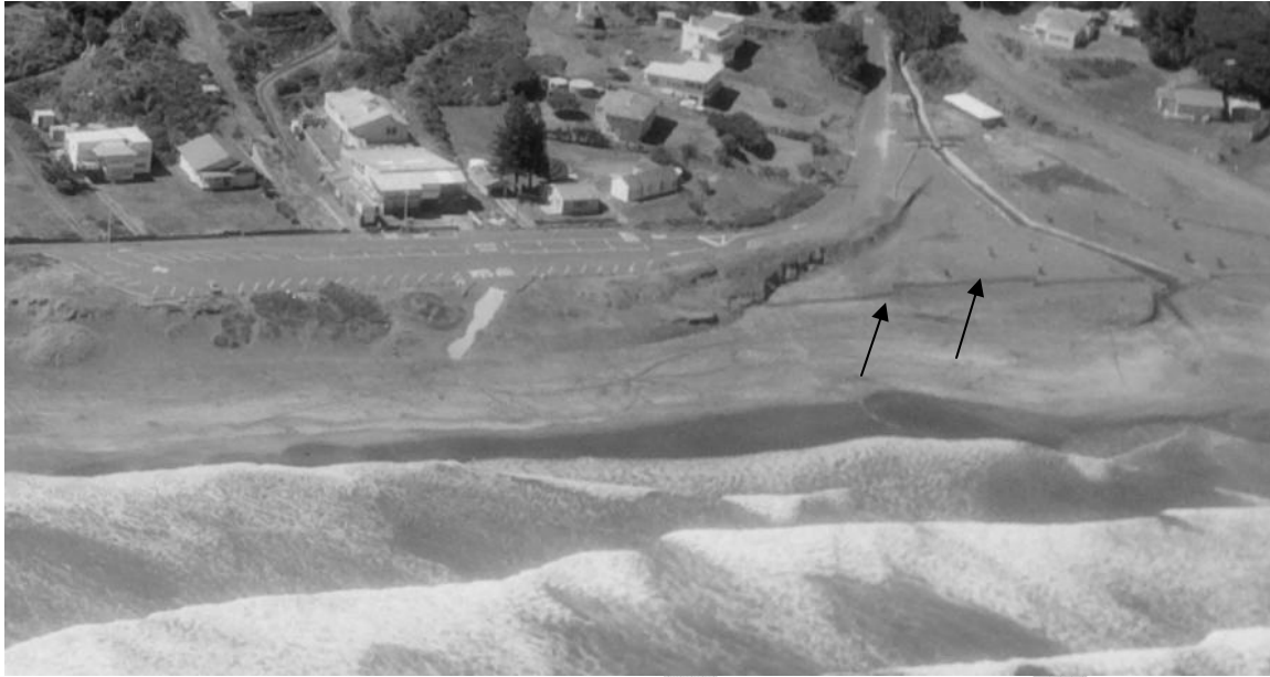
Figure 9: View of surf club car park and Moana Stream entrance area in 1985. Note the concrete stream training works in the Moana Stream and the placement of sand trapping fences (arrowed) to create dunes on the immediate northern side of the former embayment.
