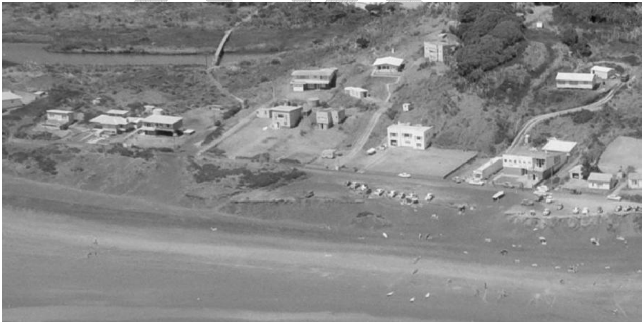
Figure 7: Photograph from 1963 showing area of Piha fronting surf club and areas to the north. Note that dunes fronting the surf club have now been levelled to create a car park and the dune face seaward of this car park is now largely devoid of vegetation. (Whites Aviation photo – from Alexander Turnbull Library).
