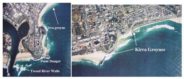
Figure 3: Aerial view of Point Danger to Kirra Point groyne at the top of the picture (left), and the 2 groynes on Kirra Point (right), Gold Coast, Australia (GOLD COAST CITY COUNCIL, 23-4-96).
