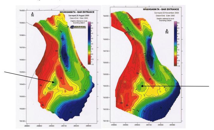
Excavation of channel, 750 m. X15m. X 1.9 recorded 32,000m3 removed.
