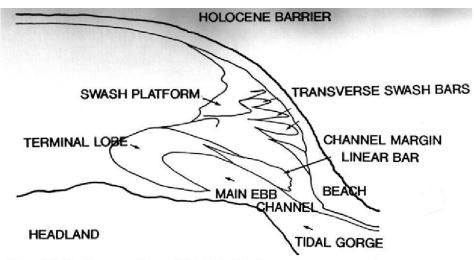
Figure 2.8: The diagrammatic form of the ebb-tidal delta.
