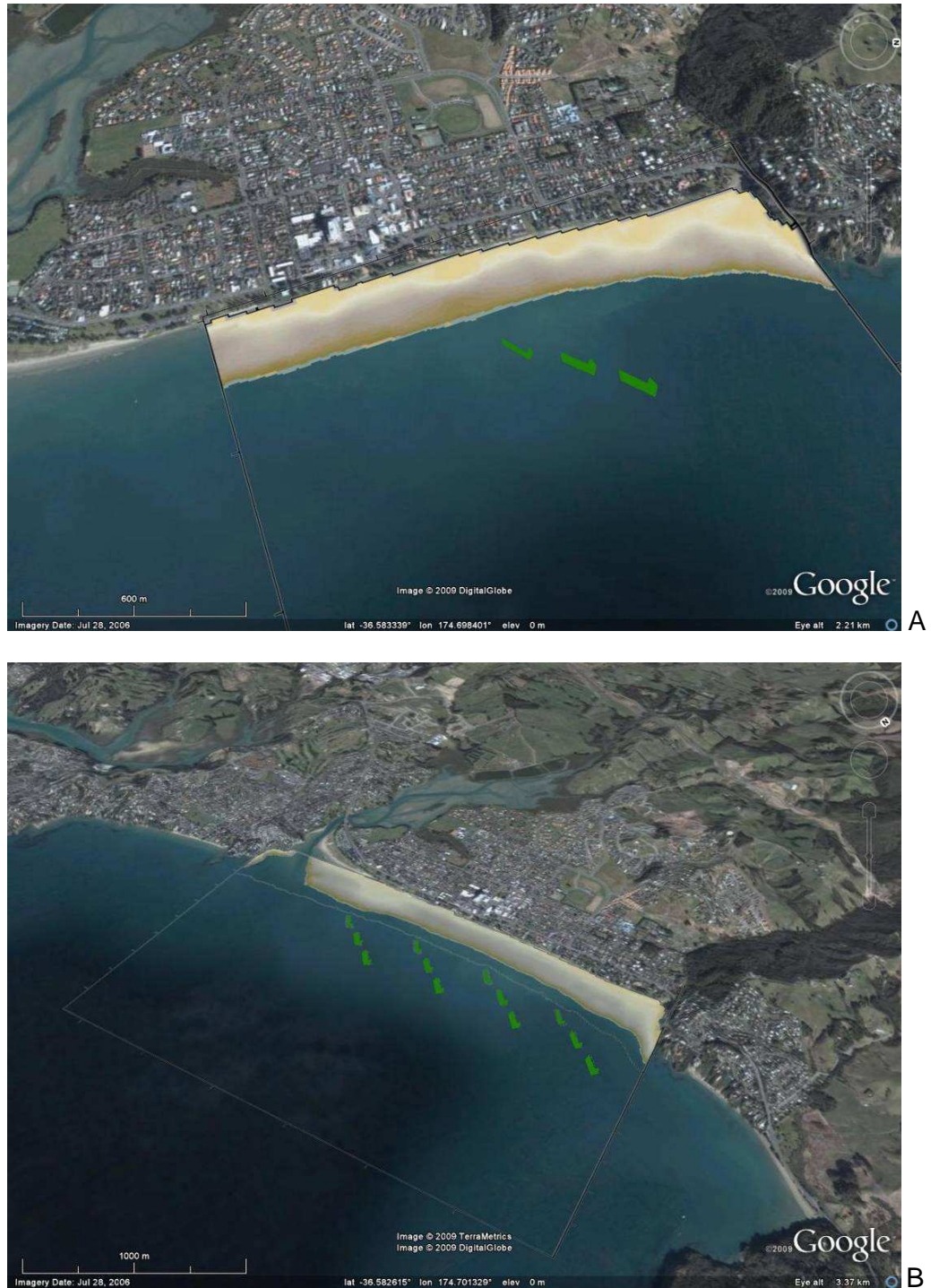
Figure 5. Views of the overall projects plan. The first of four reef systems located on the northern part of the beach (A). The larger master plan of 4 reef systems along the length of Orewa Beach is shown in B. Outputs extracted from model simulations with tide at 1.0 m above CD – the transition from grey to sand in panel A is the approximate high tide mark.
