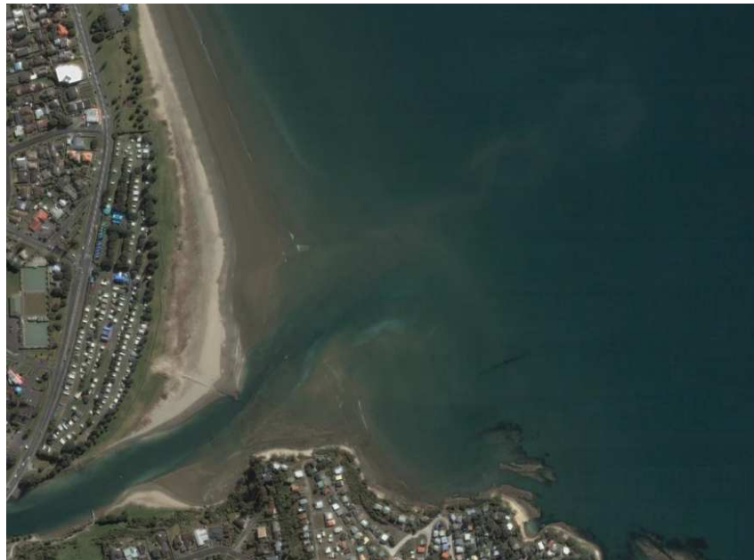
Figure 2.37. Google Earth image showing the variable eddies moving out over the ebb tidal delta (31 August 2004). Such eddies result in unsteady currents as seen in Figure 2.33, which are not replicated in a 2-dimensional model.
