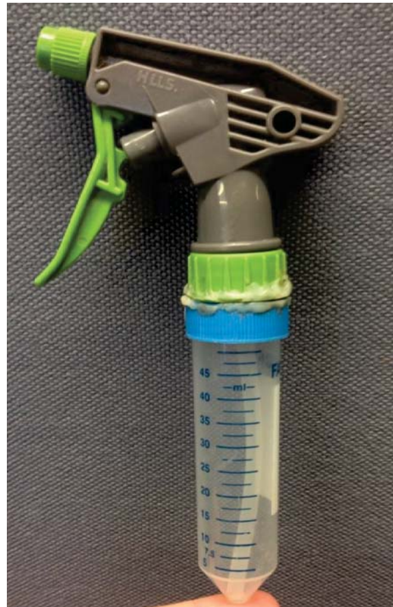
Photo 3.1: Modified spray bottle used to apply additional 'rainfall'.
