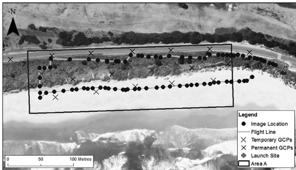
Figure 5. The flight path and GCP layout for flight one at St. Kilda Beach.
