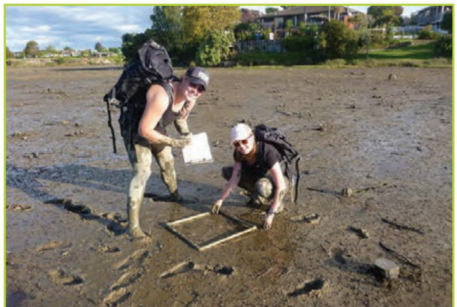
Monitoring to measure recovery of sediments and decomposition/erosion of mangrove roots (below-ground biomass) at Pahurehure Inlet, Manukau Harbour.
