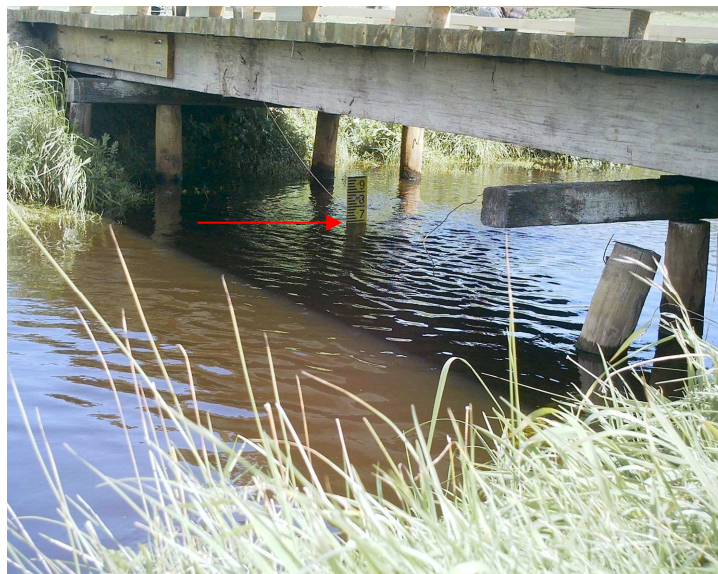
Figure 4.9 The staff gauge (with miniTROLL attached) located under the bridge at the Waikanae Golf Course. This is 73m downstream from where the Ngarara Stream emerges from the wetland.
