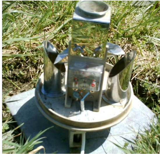
Figure 4.2 The mechanism within a 'tipping-bucket' rain gauge. This particular gauge was installed at Site 7, but was later replaced following vandalism that destroyed the gauge.
