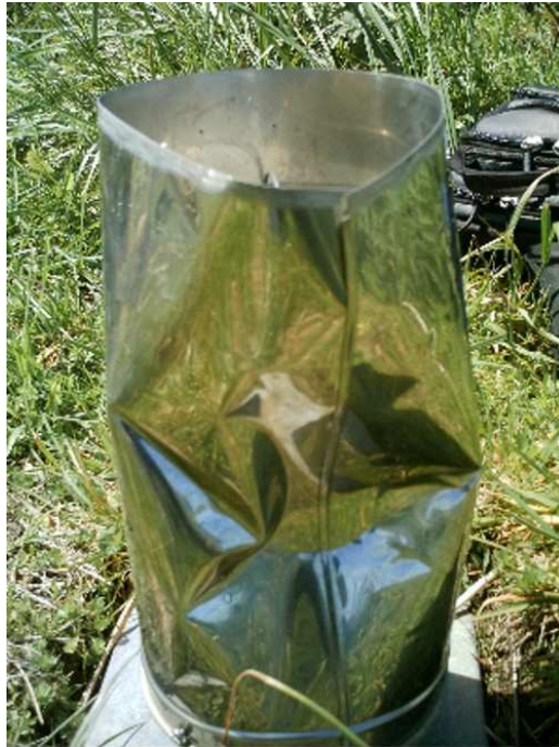
Figure 4.6 Vandalised rain gauge located at Site 7, on the edge of the Waikanae Golf Course.
