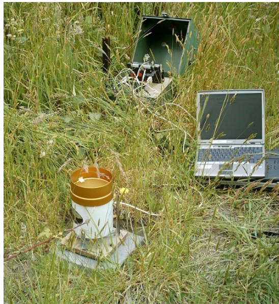
Figure 4.5 The location of the rain gauge at Site 7. Note the different type of gauge in this photograph compared to Figure 4.2 . The gauge was changed 3 months into data collection because of to vandalism to original gauge.
