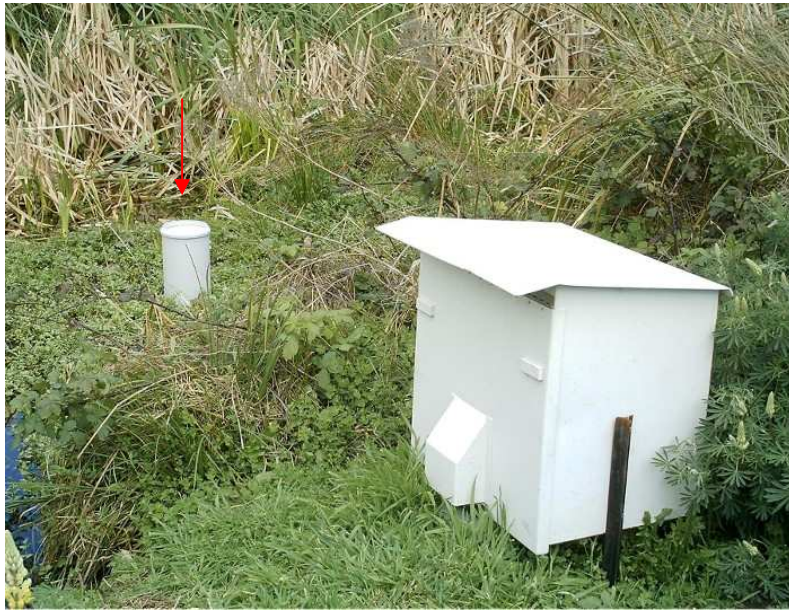
Figure 4.4 The location of the monitoring equipment located at Site 4. The rain gauge can be seen (red arrow). The site also has TDR probes that are located underground just beyond the scope of the photograph near the warratah that supports the data logger housing.
