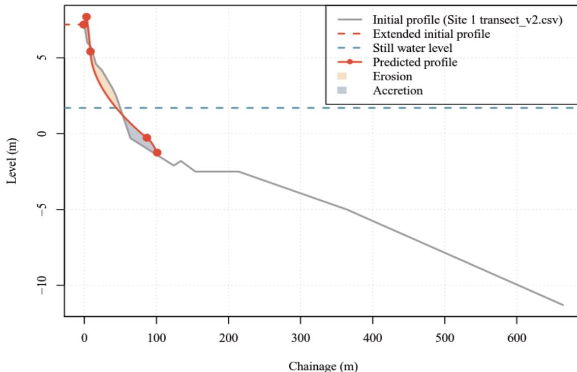
Figure 11: Modelled profile change using the empirical model Shingle-B
