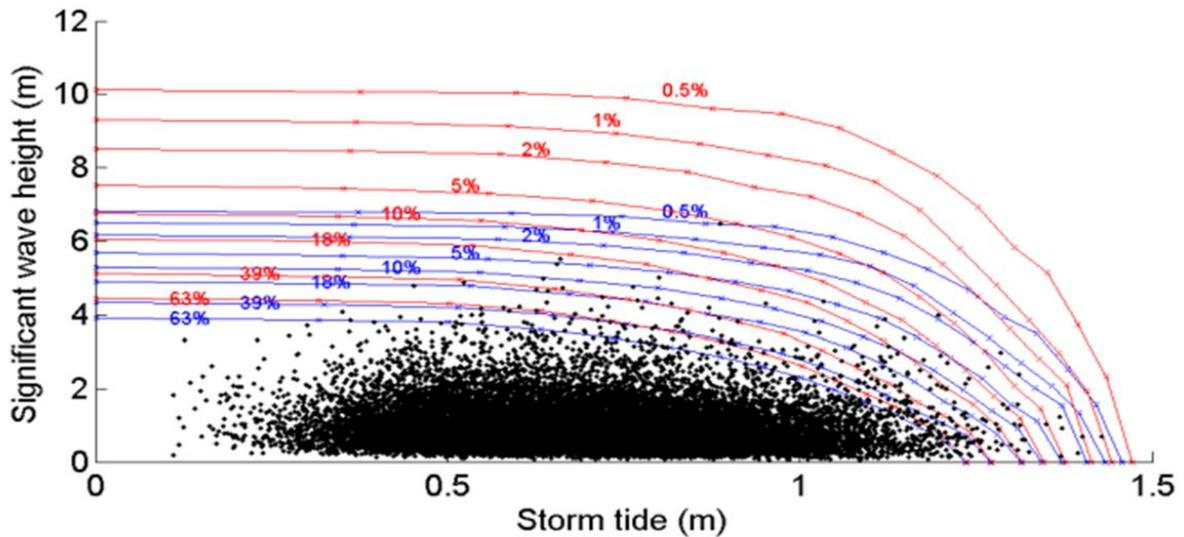
Figure 7 Joint probability of significant wave height and storm tide in terms of MLOS at JP3 north of Kaikōura including model results (blue lines) and scaled results (red lines). (Source: NIWA, 2015)
