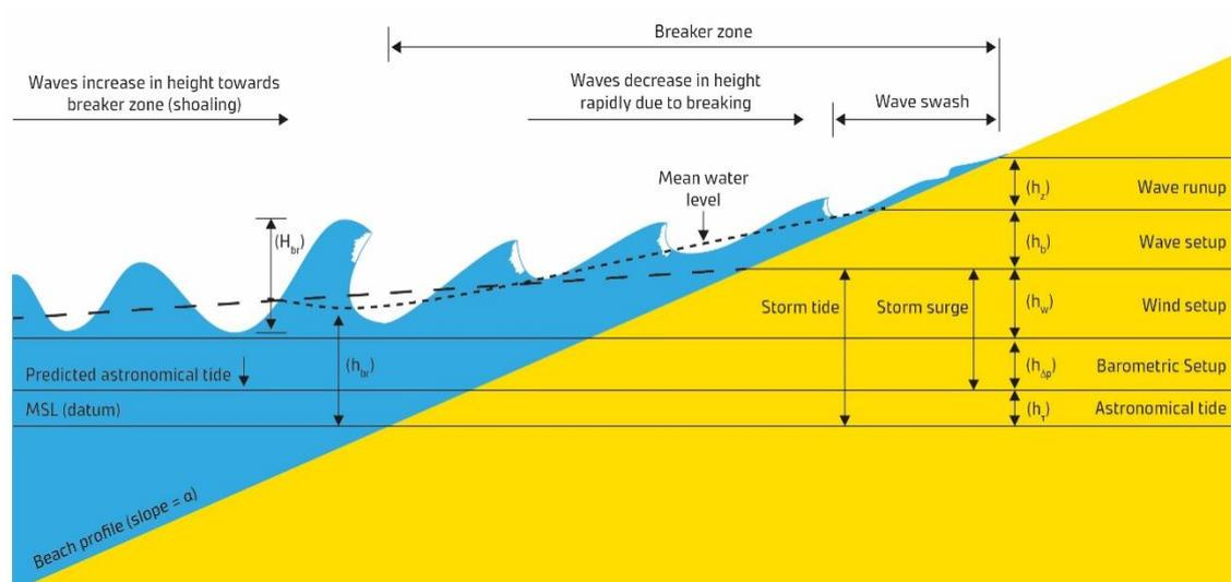
Figure 3 Schematic illustrating sources of coastal-storm inundation
