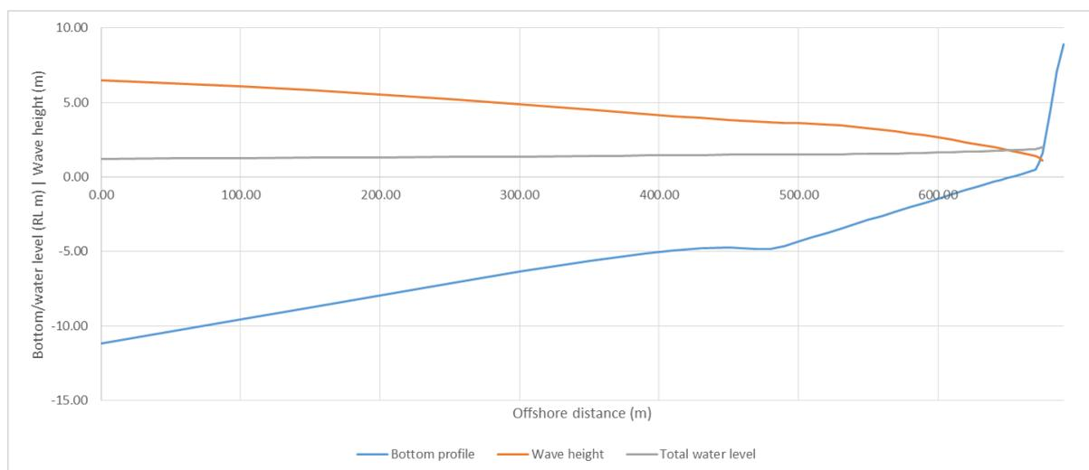
*Figure 9 Example of Unibest-LT output showing cross-shore wave height and water level transformation*
