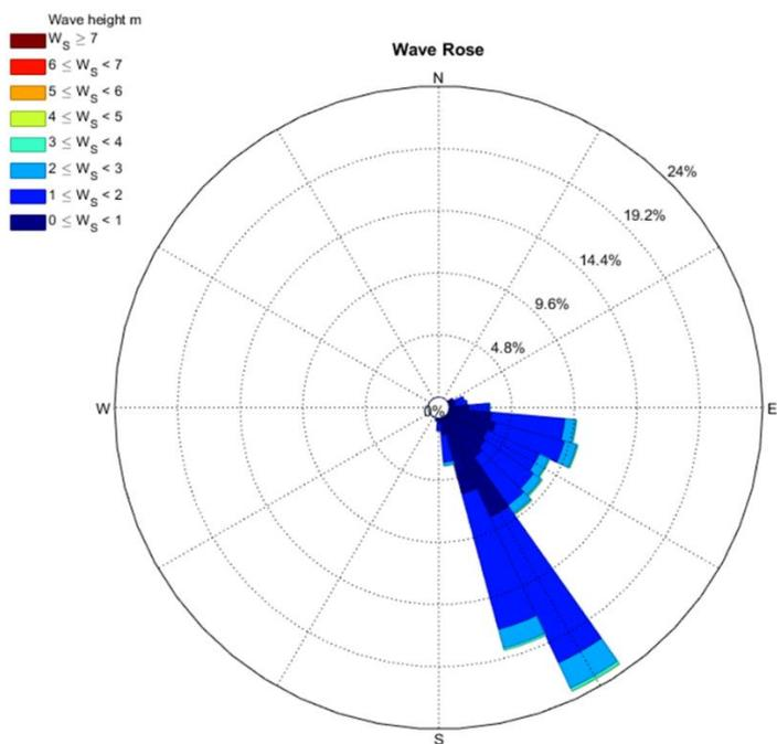
Figure 5 Wave rose showing wave height and direction at output node 173.837E, 42.254S (Source: MSL)
