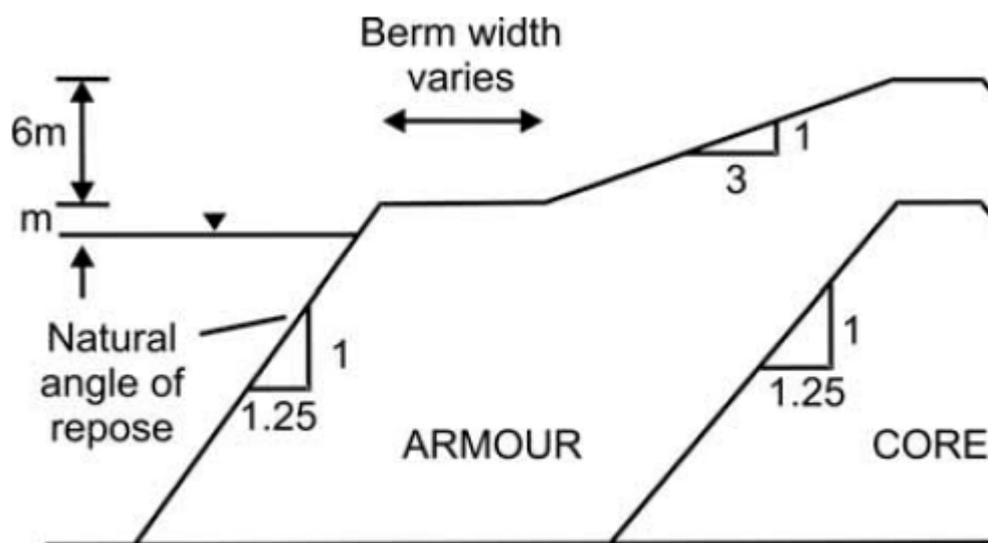
Figure 14 Typical features of a berm breakwater (Source: CIRIA/CUR C683, 2007)
