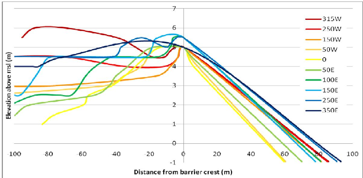
**Figure 2.4b: Beach profiles at Charlies Bay - lagoon on the left and ocean on the right (data from Environment Southland).**
