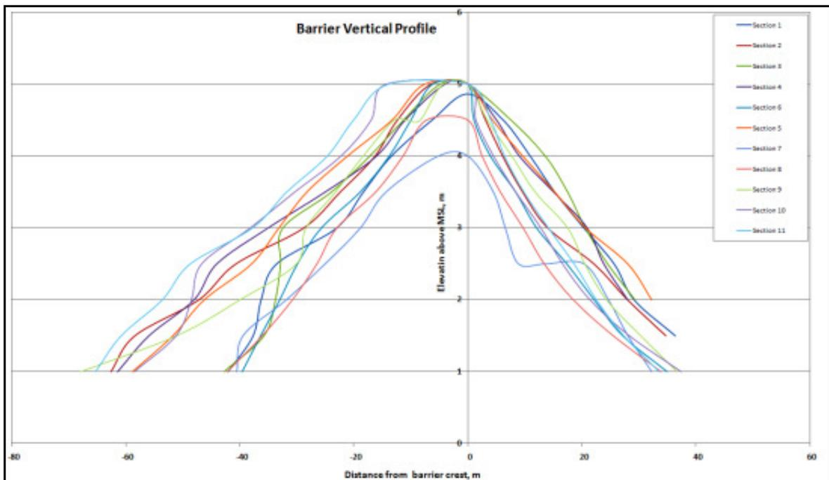
Figure 2.3b: Cross sectional profiles East and West end of Lagoon – lagoon on the left and ocean on the right (data from Environment Southland).
