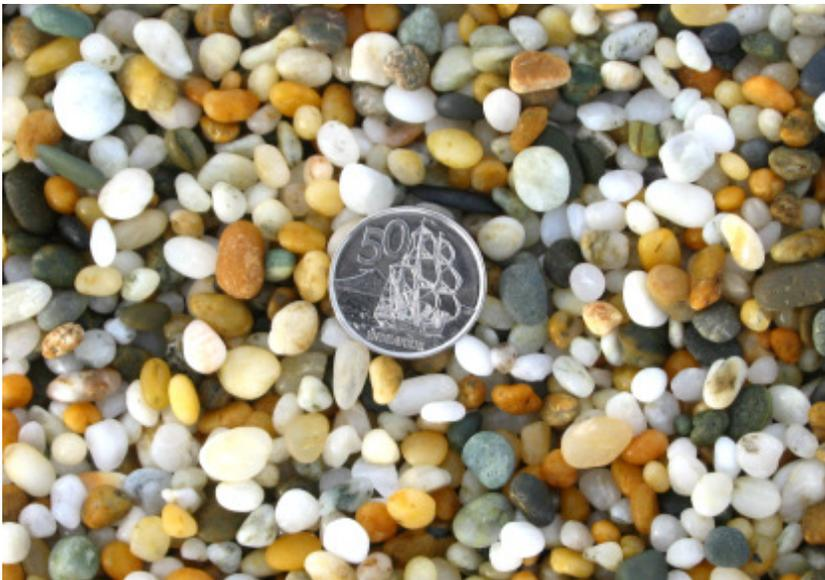
**Figure 2.1: Typical beach surface material – 6 to 8 mm median diameter gravel of variable depth.**
