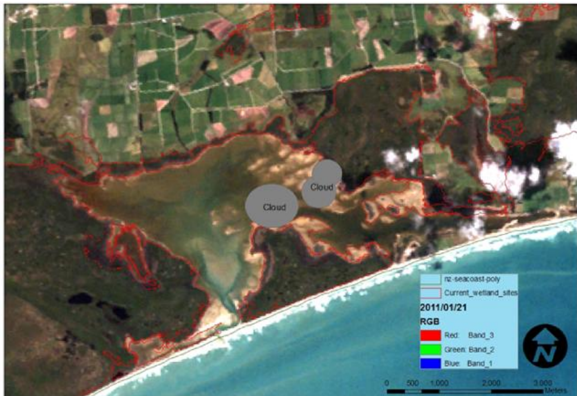
Figure 49: True colour composite of bands 1, 2, 3 (B,G,R) of Landsat on 21 January 2011. Grey boxes are used to mask some small areas of cloud.
