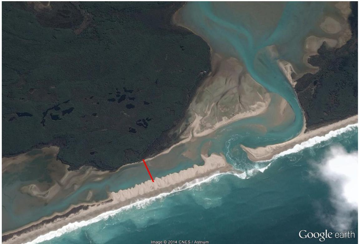
Figure 3-23 Alternative possible location for internal dike for more western Walker's Bay opening. The breach shown on the Google image would instead be to the west of the indicated location of a structure.
