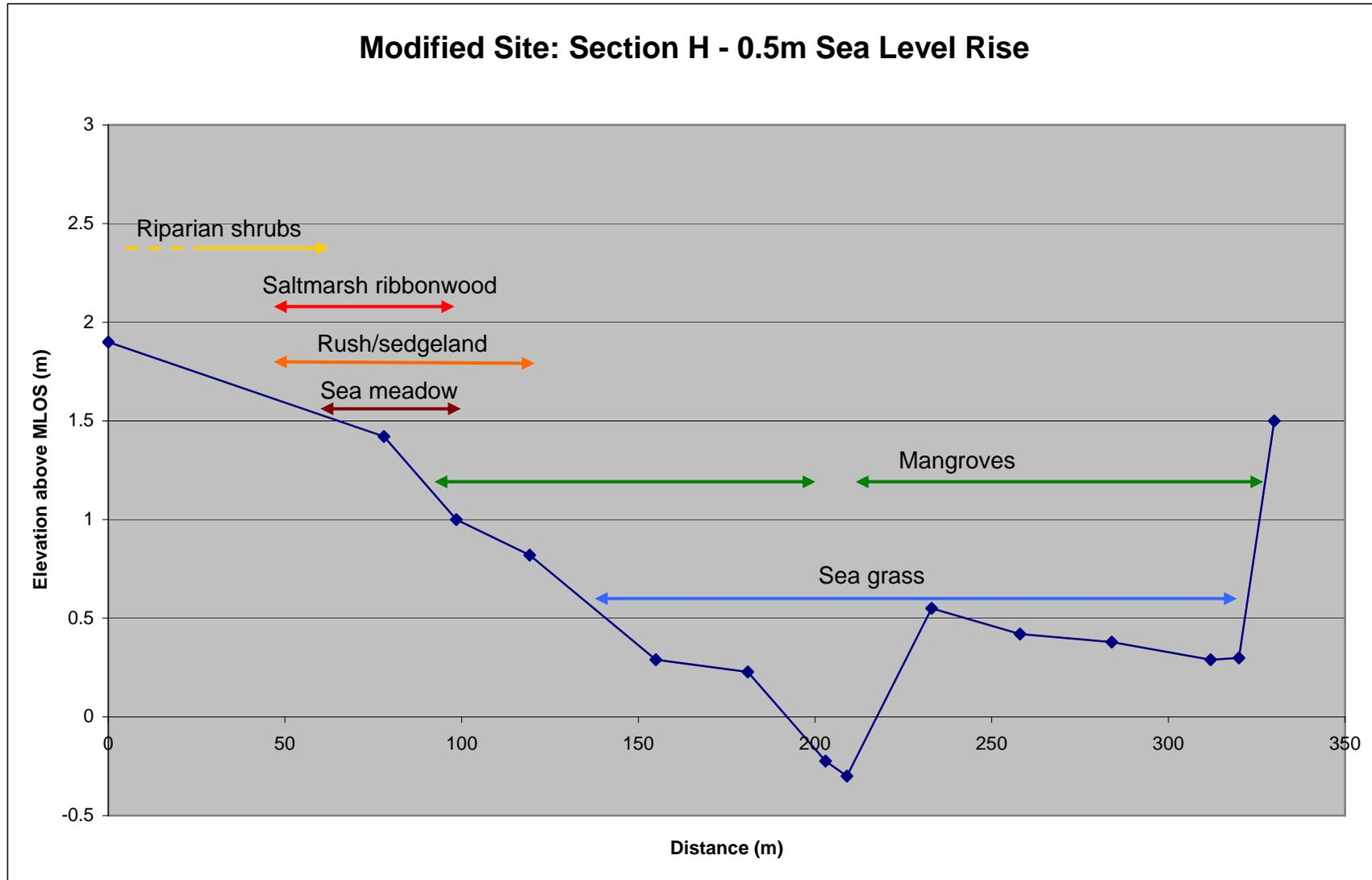
Figure 25: Typical cross-section of Modified Site (see Figure 5 for location) – 0.5 m sea level rise scenario (with flap-gate removed)
