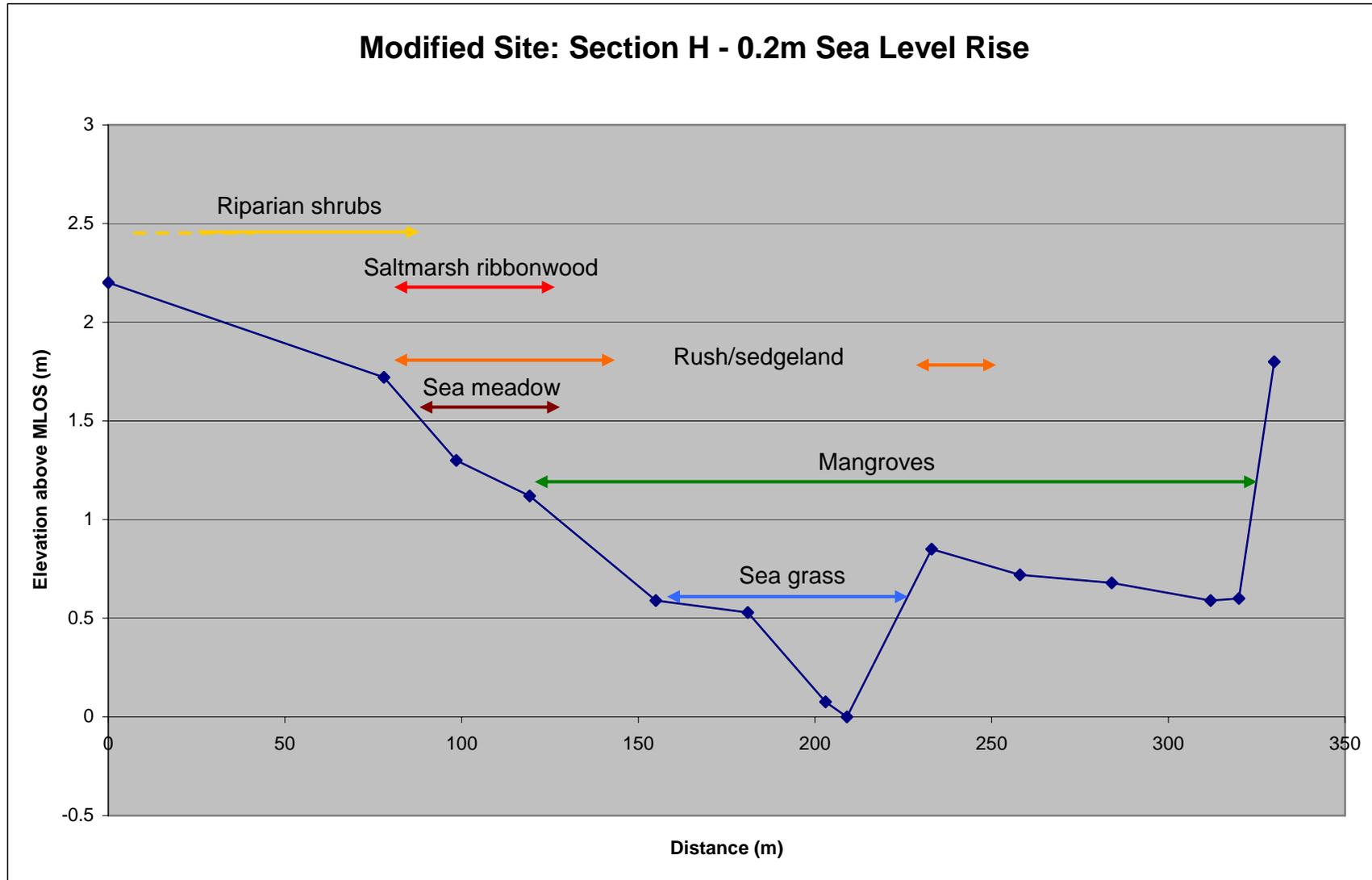
Figure 24: Typical cross-section of Modified Site (see Figure 5 for location) – 0.2 m sea level rise scenario (with flap-gate removed)
