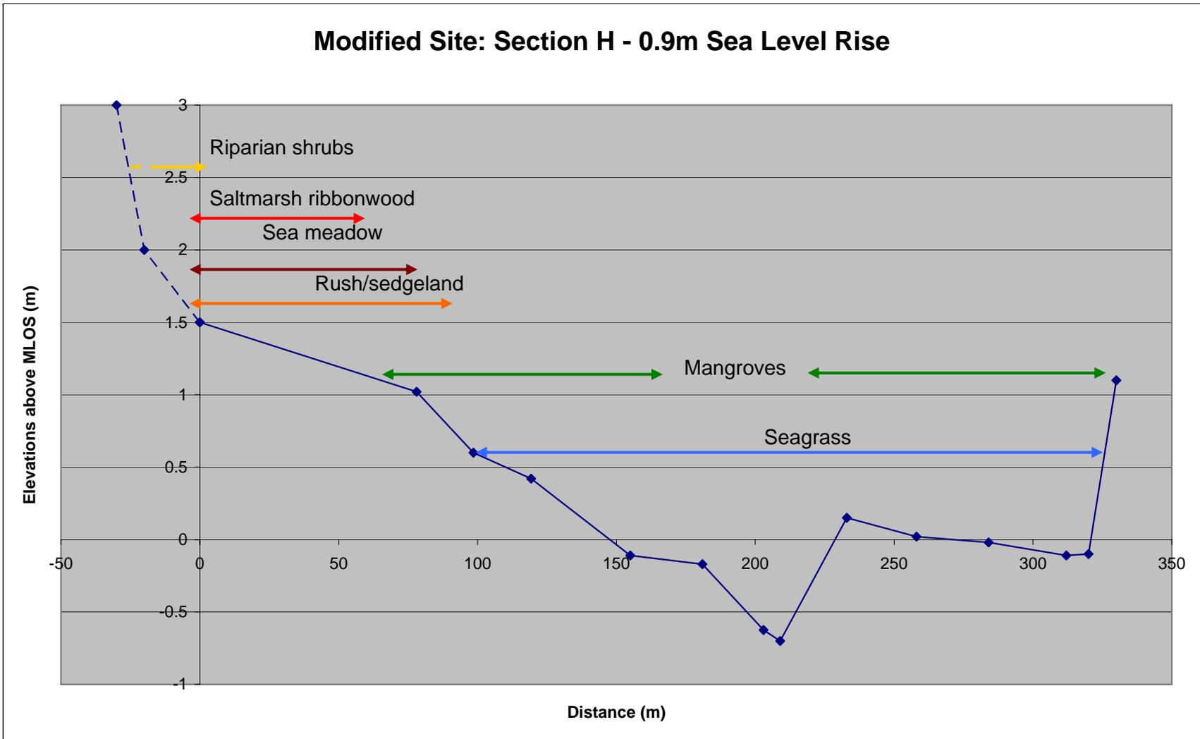
**Figure 26: Typical cross-section of Modified Site (see Figure 5 for location) – 0.9 m sea level rise scenario (with flap-gate removed)**
