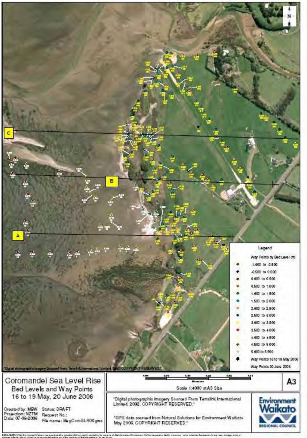
**Figure 3: Exposed Area – surveyed bed levels and locations of cross-sections**
