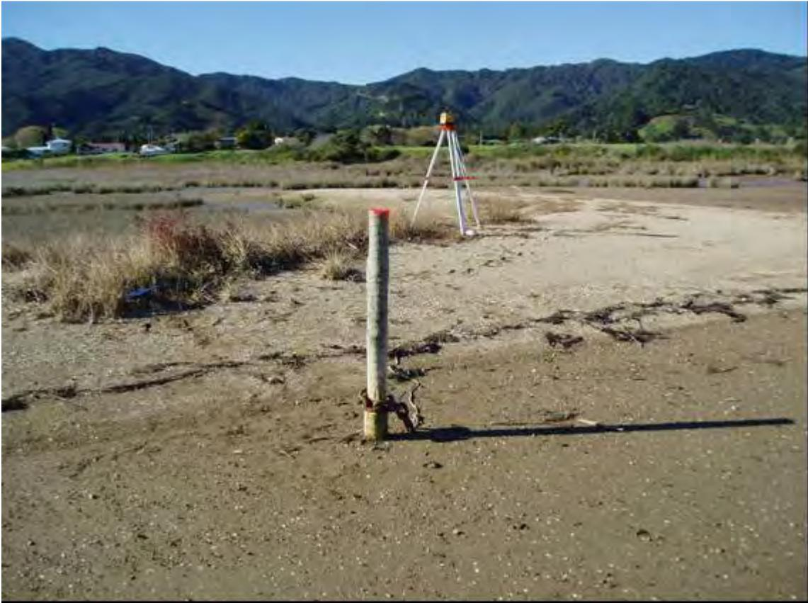
**Figure 2: A typical surveying set up used to establish local estuarine vegetation boundaries and bed levels**
