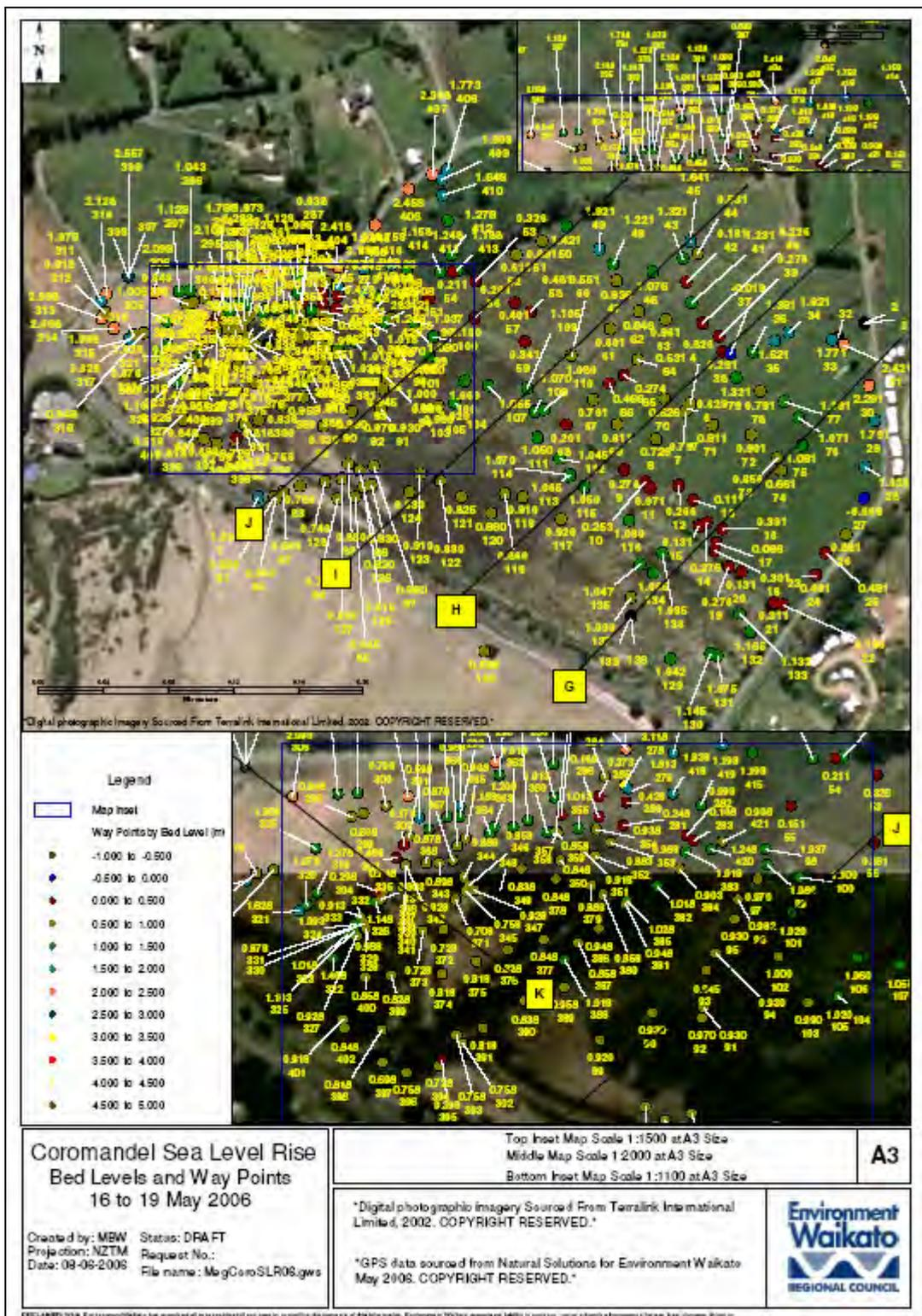
Figure 5: Modified Area – surveyed bed levels and locations of cross-sections
