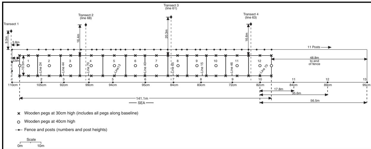
**Figure 9: Location of transects and pegs for monitoring changes in sand level on a reshaped foredune, Oakura Beach, New Plymouth.**
