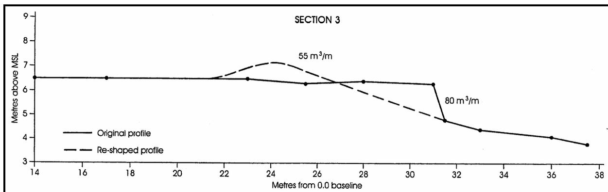
**Figure 3:** The aim with reshaping the dune at Oakura Beach was to change the original steep foredune profile to an approximately  $18^\circ$  slope extending 10 m wide on which a dense cover of native sand-binding species could be established (from Hesp and Grant 2000).
